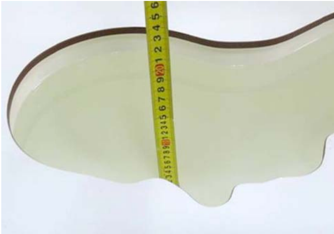
Picture 11: Liquid depth in the head Phantom (2600 MHz, 15.4cm depth)
