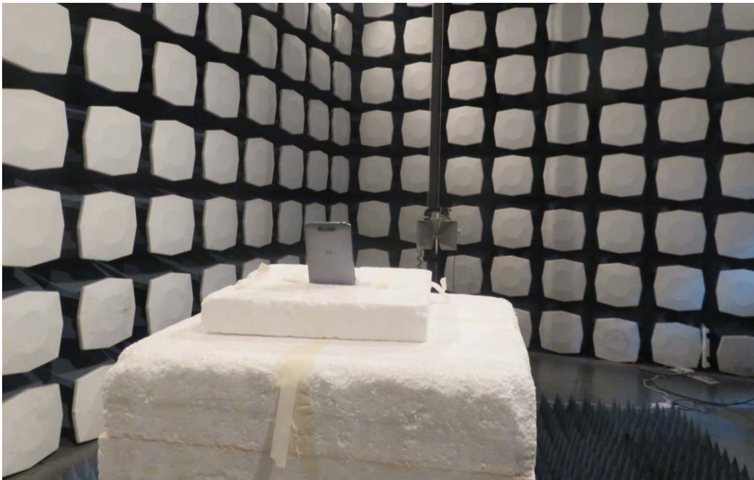
Picture 2: Radiated Spurious Emissions Test setup
