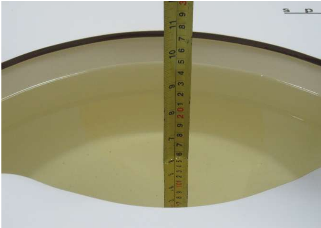
Picture D 13: Liquid depth in the flat Phantom (750MHz) (15.3cm deep)
