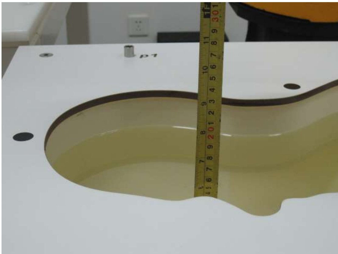
Picture D 12: Liquid depth in the head Phantom (750MHz) (15.4cm deep)
