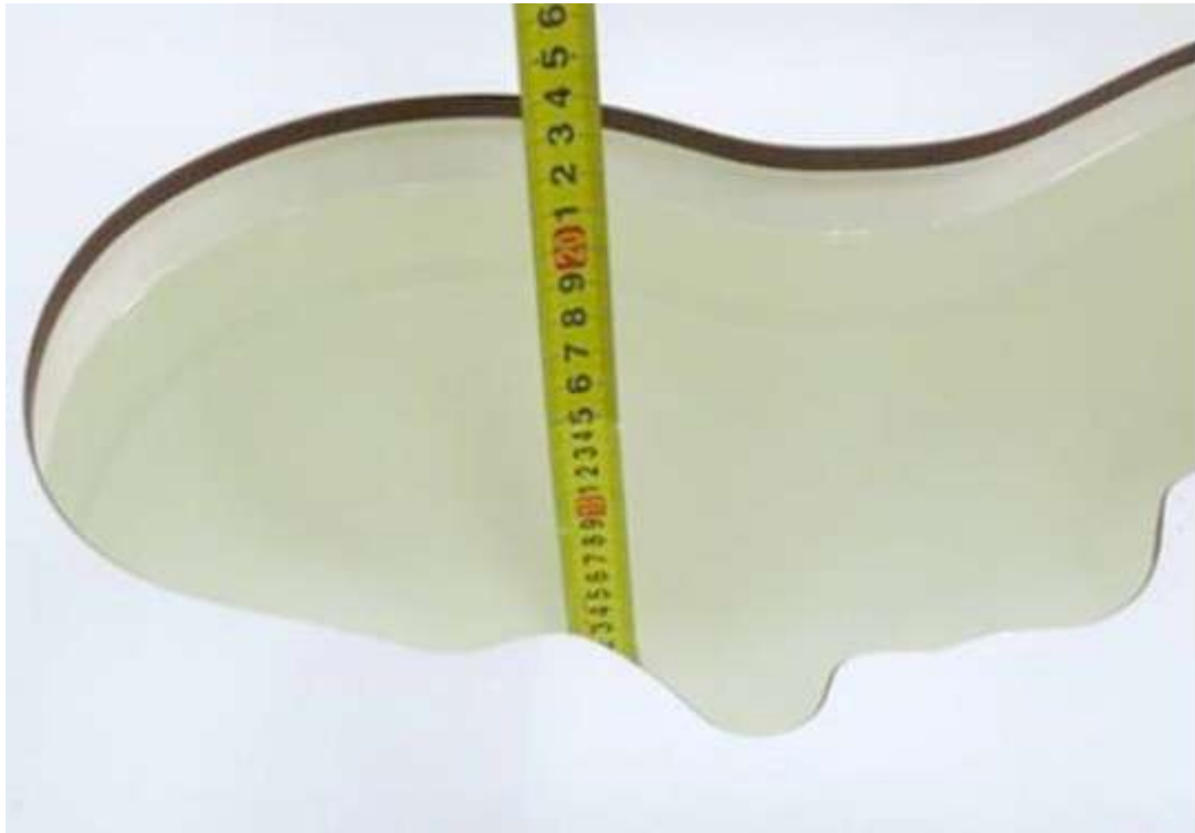
Picture C.11: liquid depth in the head Phantom (2600 MHz) (15.3cm deep)
