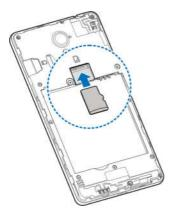
Insert the battery by aligning the metal contacts on the battery with the metal contacts in the battery compartment. Gently push down on the battery until it locks into place.
