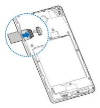
3. Hold your microSDXC card with the metal contacts facing down and slide it into the microSDXC card slot.
