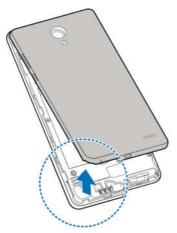
Hold the micro-SIM card with its cut corner oriented as shown and slip it into the card holder.
