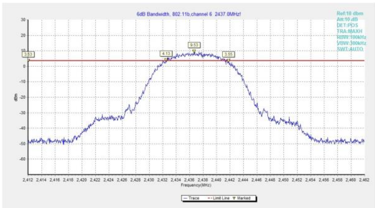
Fig.A.4.2 Occupied 6dB Bandwidth (802.11b, Ch 6)
