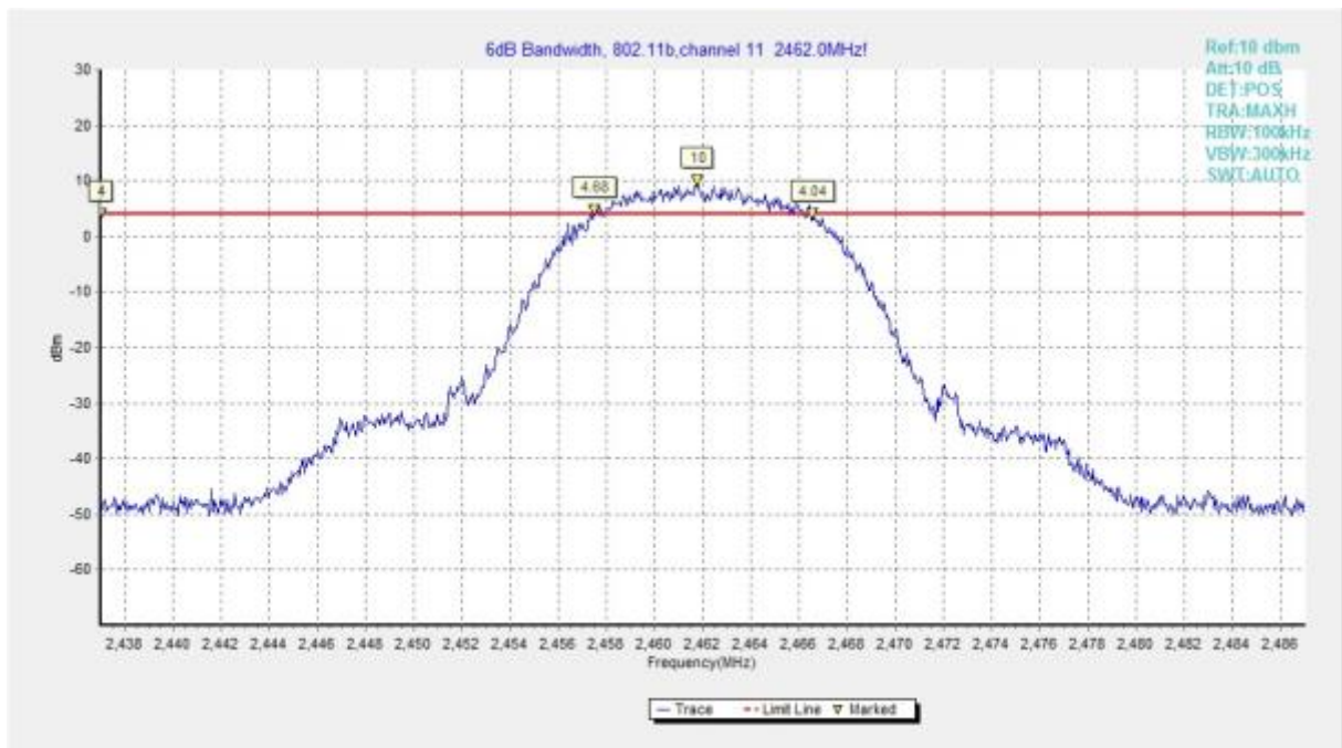
Fig.A.4.3 Occupied 6dB Bandwidth (802.11b, Ch 11)
