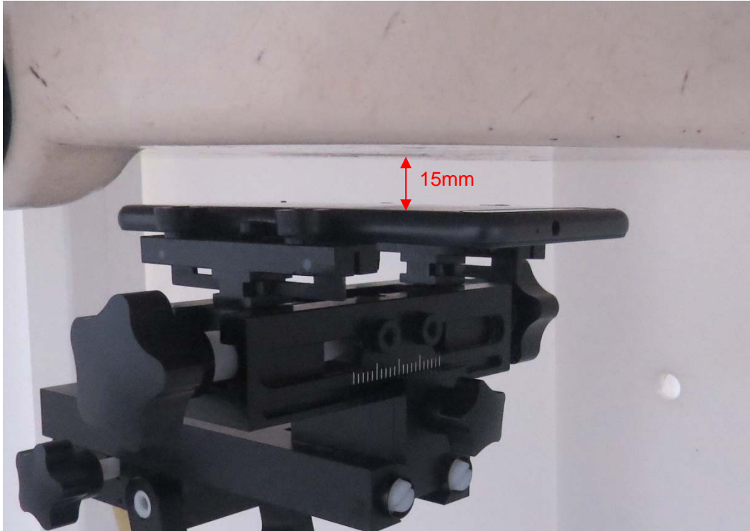
Picture 5: Back Side, the distance from handset to the bottom of the Phantom is 15mm
