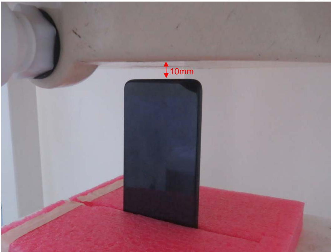
Picture 12: Bottom Side, the distance from handset to the bottom of the Phantom is 10mm
