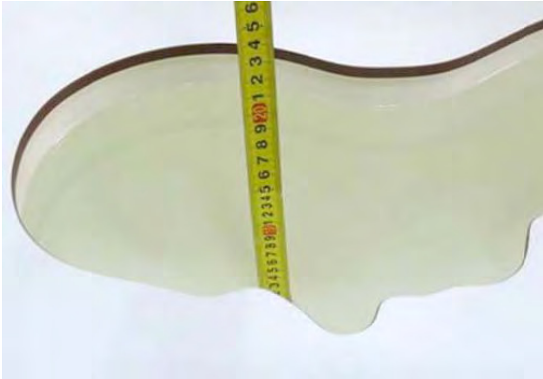
Picture 7: liquid depth in the head Phantom (1750 MHz, 15.3cm depth)
