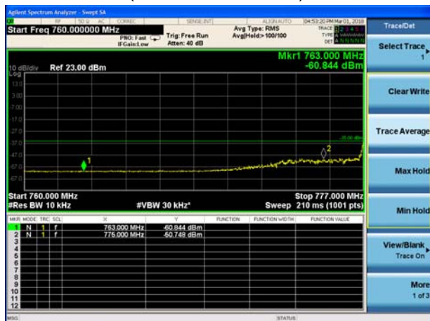
LTE Band 13 QPSK 5MHz CH-Low, 100%RB (763MHz ~775MHz)
