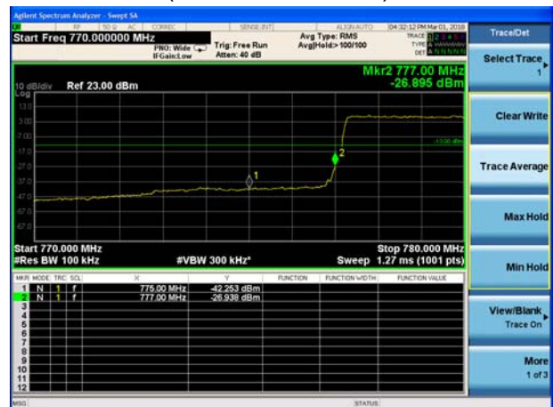
LTE Band 13 QPSK 5MHz CH-Low, 100%RB (775MHz ~777MHz)
