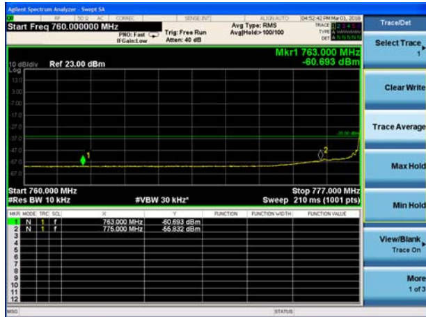
LTE Band 13 QPSK 5MHz CH-High, 1 RB (787MHz ~793MHz)
