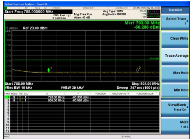
LTE Band 13 QPSK 5MHz CH-Low, 100%RB (775MHz ~777MHz)
