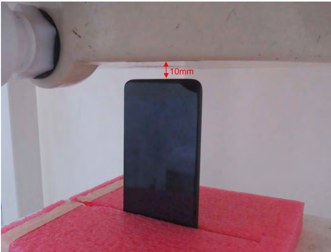
Picture 27: Bottom Side, the distance from handset to the bottom of the Phantom is 10mm
