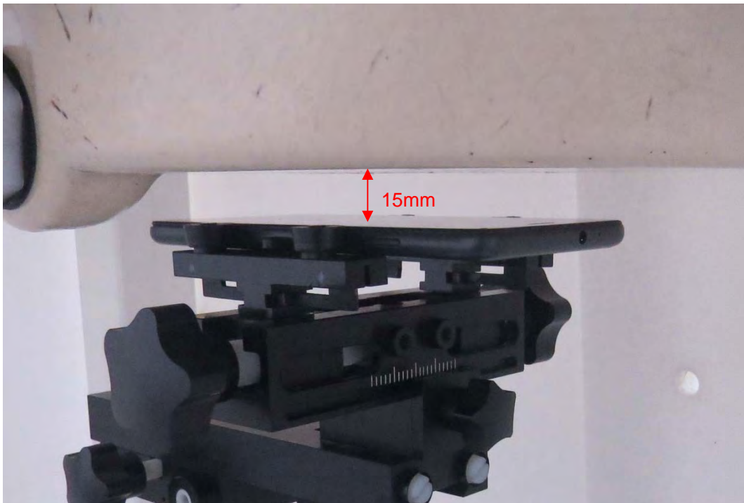
Picture 21: Front Side, the distance from handset to the bottom of the Phantom is 15mm
