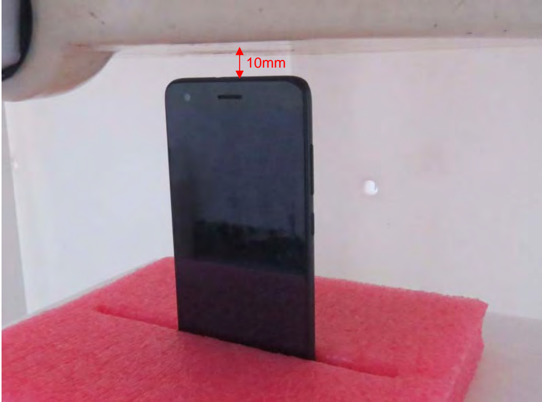
Picture 26: Top Side, the distance from handset to the bottom of the Phantom is 10mm
