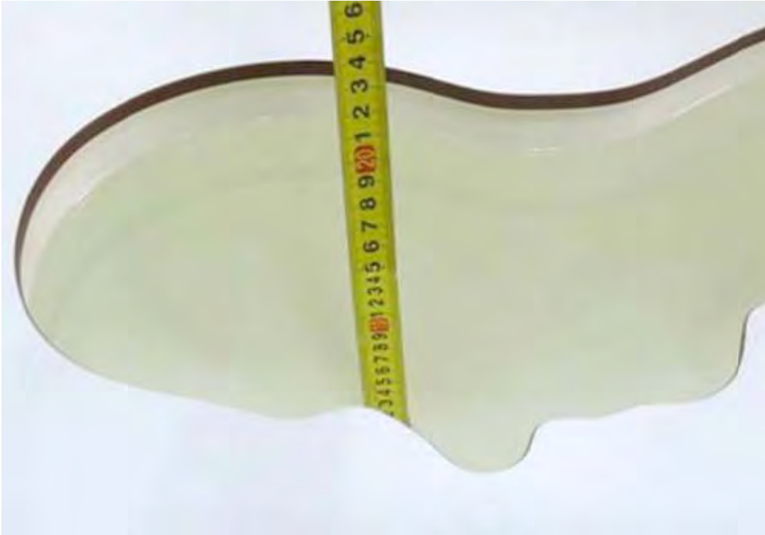
Picture 13: Liquid depth in the head Phantom (2600 MHz, 15.4cm depth)
