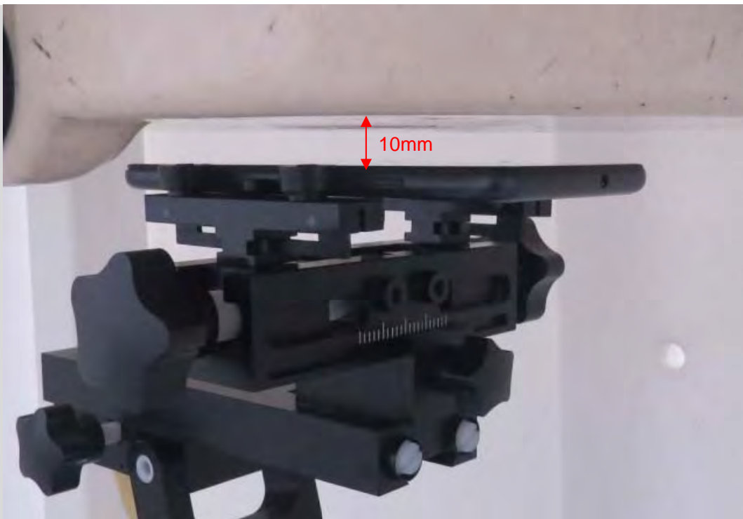
Picture 23: Front Side, the distance from handset to the bottom of the Phantom is 10mm
