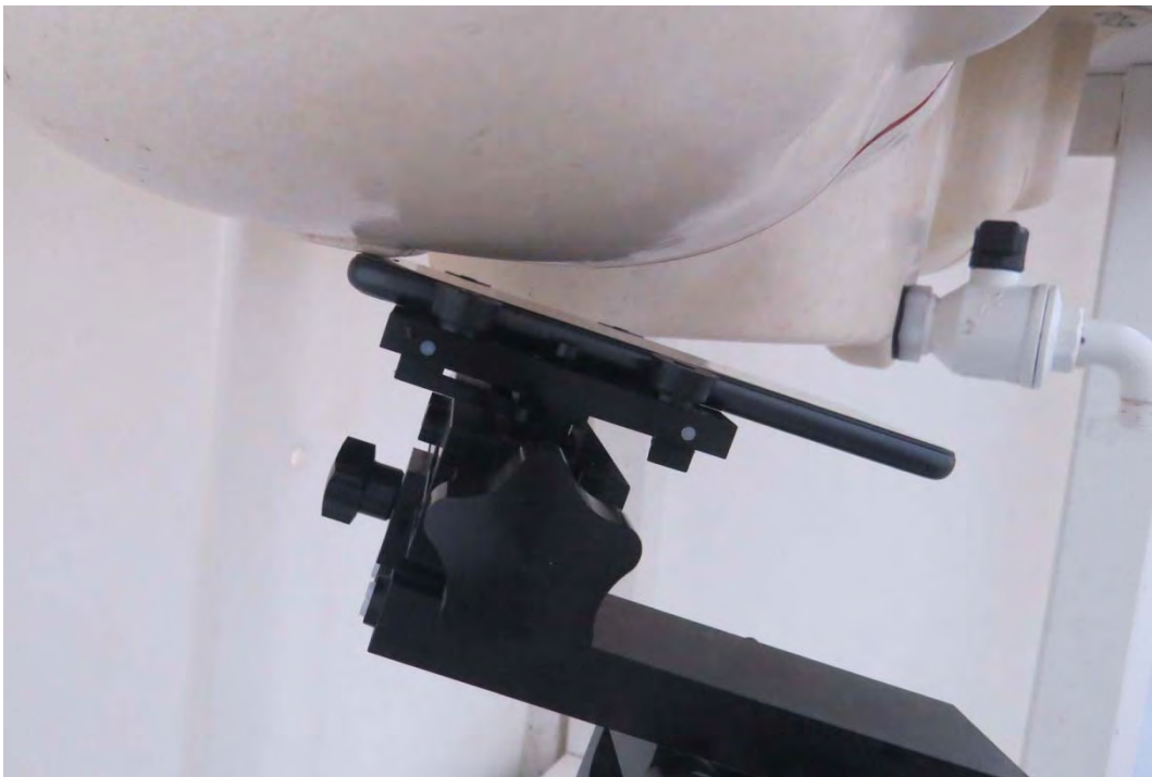
Picture 19: Right Hand Tilt 15 Degree Position
