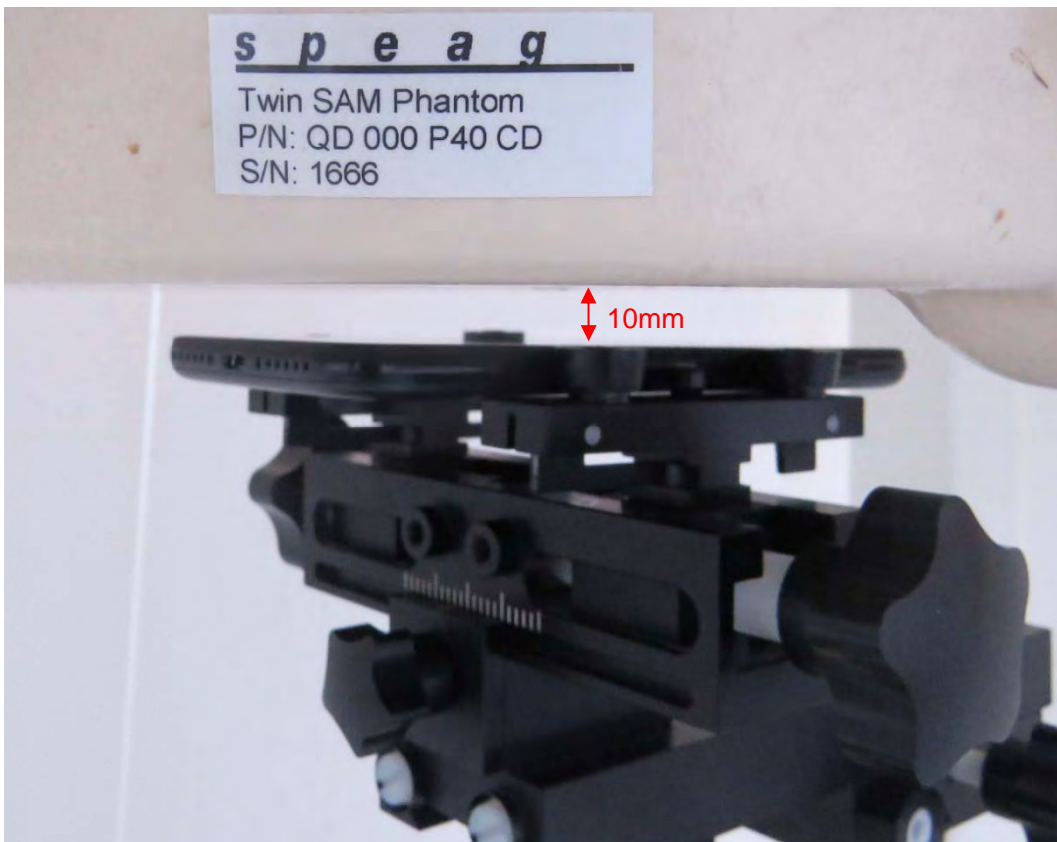
Picture 21: Front Side, the distance from handset to the bottom of the Phantom is 10mm
