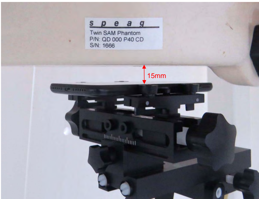
Picture 19: Front Side, the distance from handset to the bottom of the Phantom is 15mm
