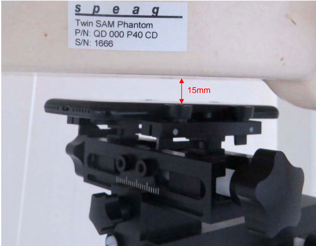
Picture 18: Back Side, the distance from handset to the bottom of the Phantom is 15mm
