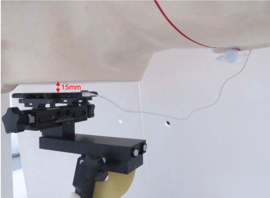
Picture 26: Back Side with Earphone 1, the distance from handset to the bottom of the Phantom is 15mm
