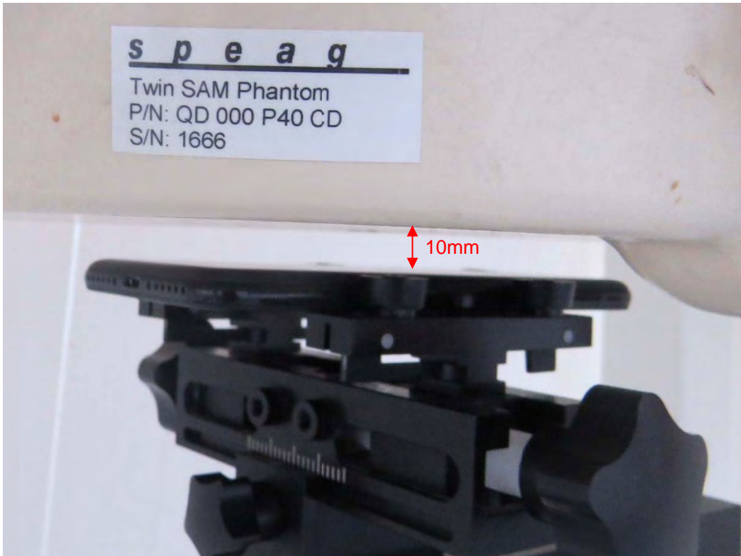
Picture 20: Back Side, the distance from handset to the bottom of the Phantom is 10mm
