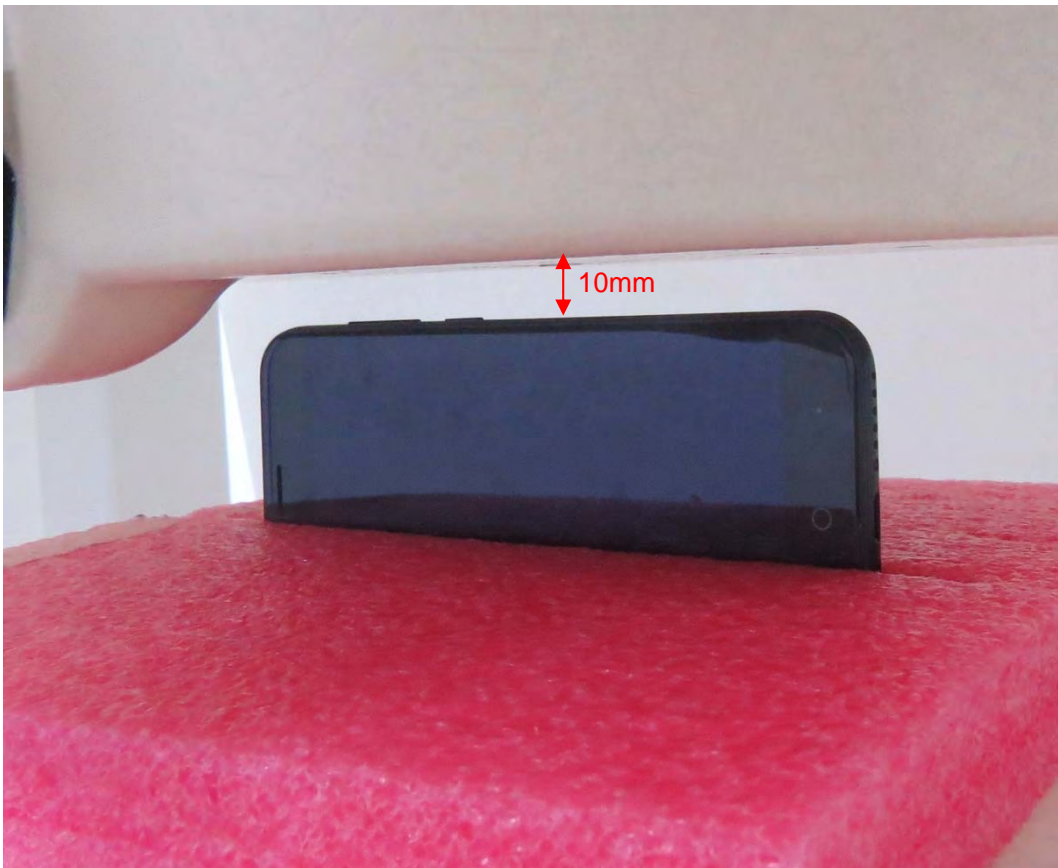
Picture 23: Right Side, the distance from handset to the bottom of the Phantom is 10mm
