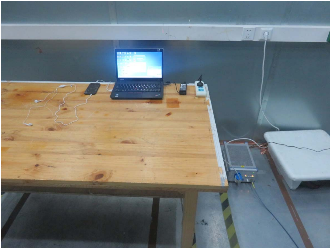
Picture 3 Conducted Emission Test Setup
