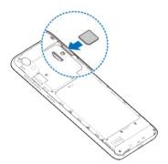
Hold your microSDXC card with the metal contacts facing down and slide it into the microSDXC card slot.
