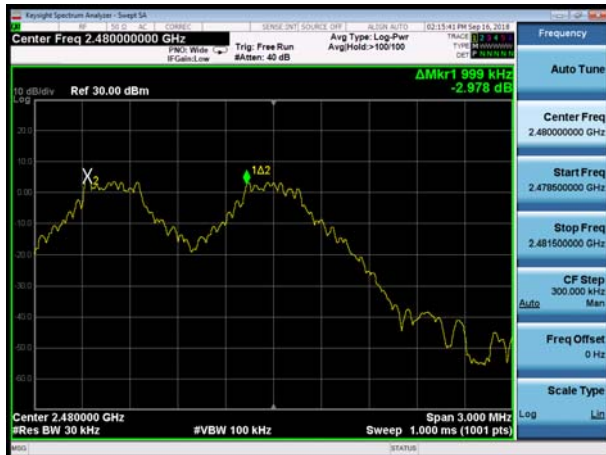
BT DH5 CH78, Carrier frequency (MHz): 2480
