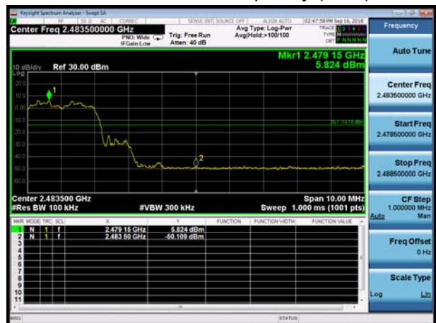
BT 3DH5 CH78, Carrier frequency (MHz): 2480
