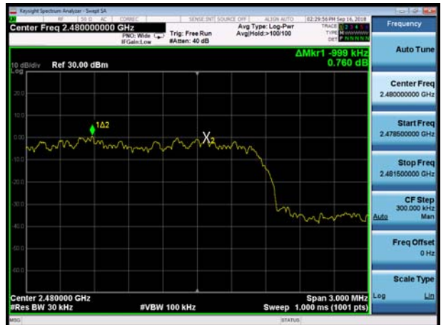
BT 2DH5 CH78, Carrier frequency (MHz): 2480
