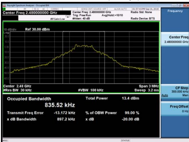
BT DH5 CH78, Carrier frequency (MHz): 2480
