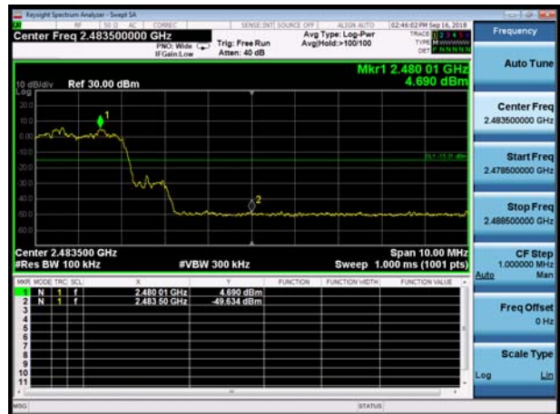
BT 3DH5 CH78, Carrier frequency (MHz): 2480
