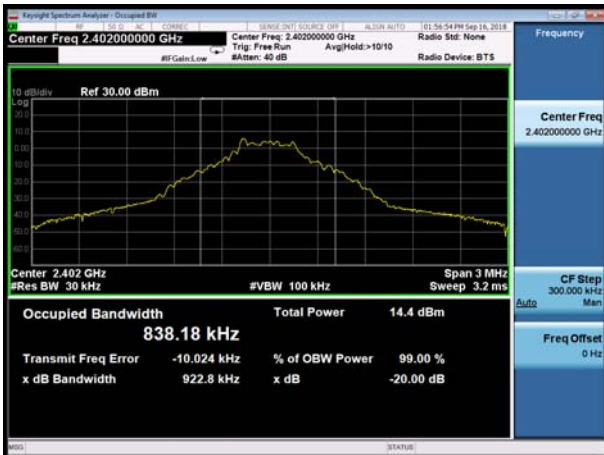
BT DH5 CH39, Carrier frequency (MHz): 2441
