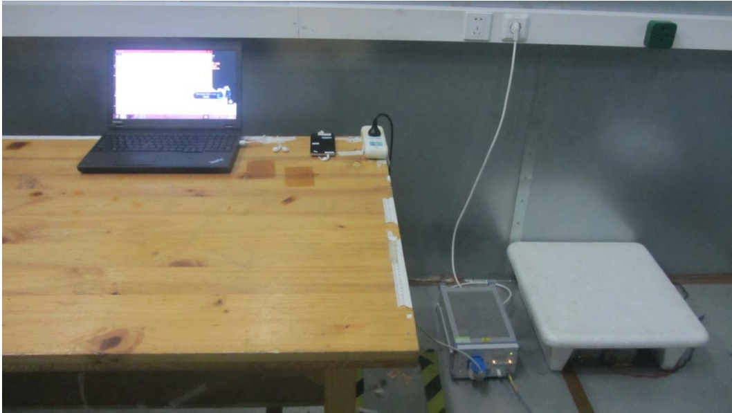
Picture 2 Conducted Emission Test Setup
