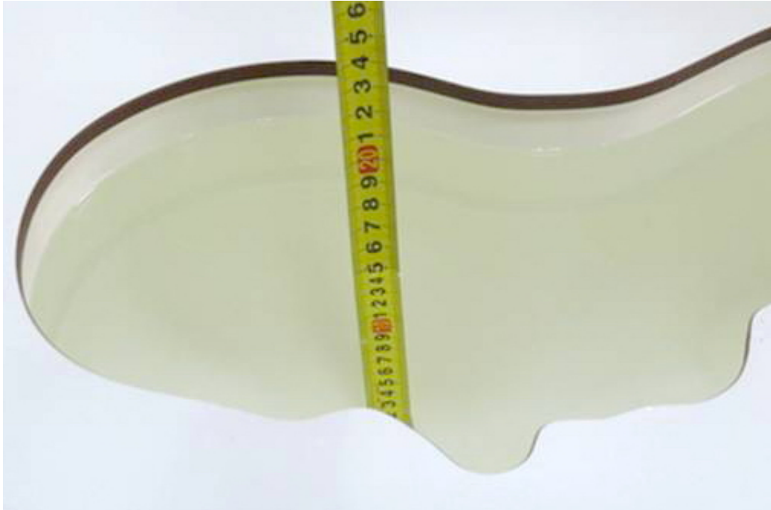
Picture 1: liquid depth in the head Phantom
