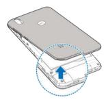
Hold the nano-SIM card with its cut corner oriented as shown and slip it into the card holder.
