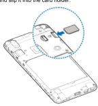
Hold your microSDXC card with the metal contacts facing down and slide it into the microSDXC card slot.
