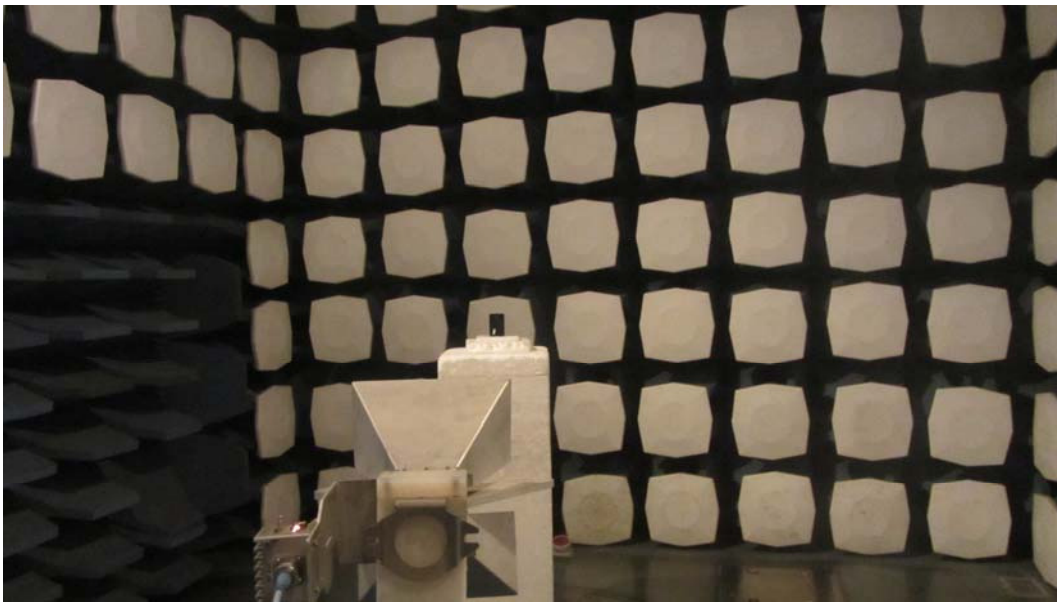
Picture 2: Radiated Spurious Emissions Test setup
