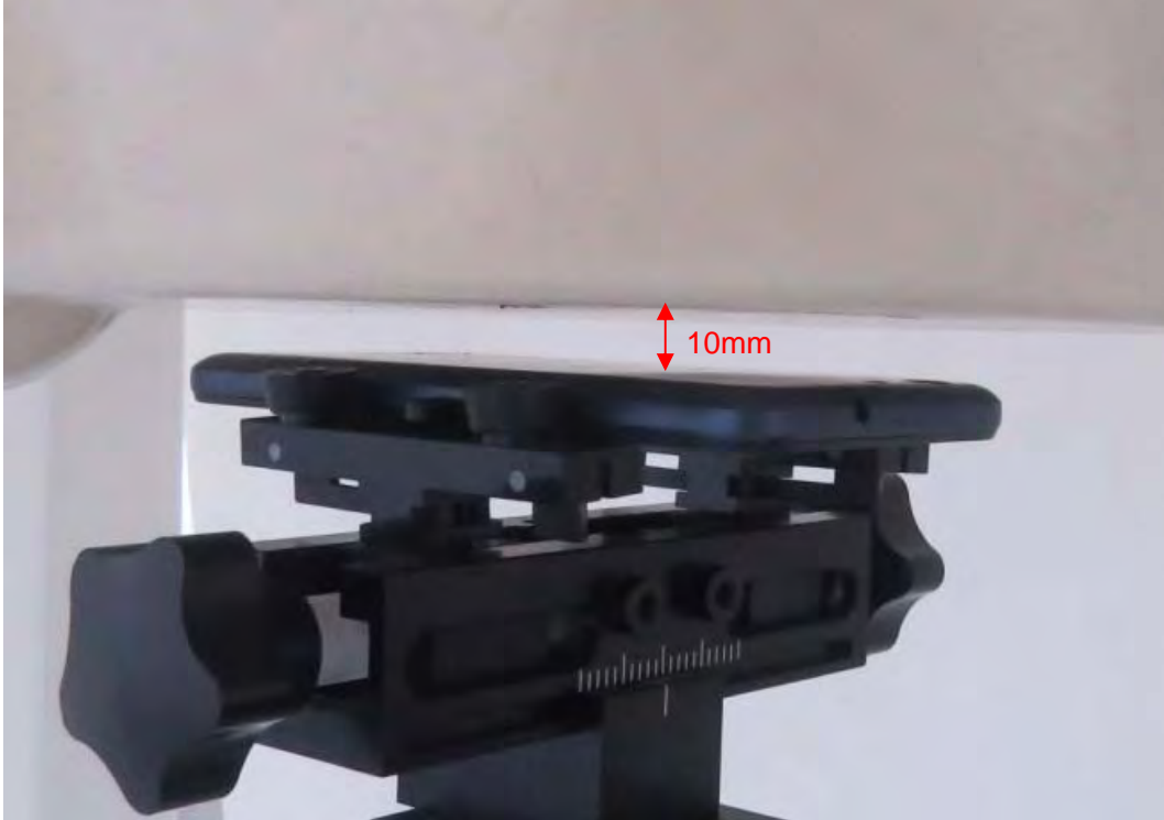
Picture 20: Back Side, the distance from handset to the bottom of the Phantom is 10mm
