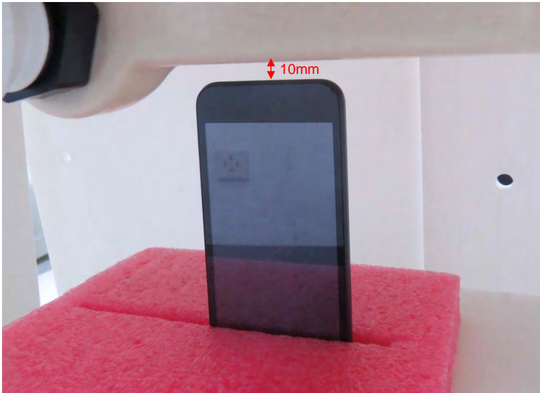
Picture 25: Bottom Side, the distance from handset to the bottom of the Phantom is 10mm
