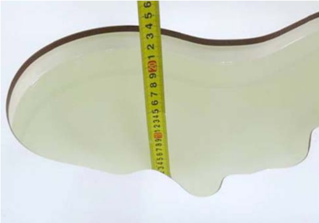
Picture 5: liquid depth in the head Phantom (1750 MHz, 15.3cm depth)
