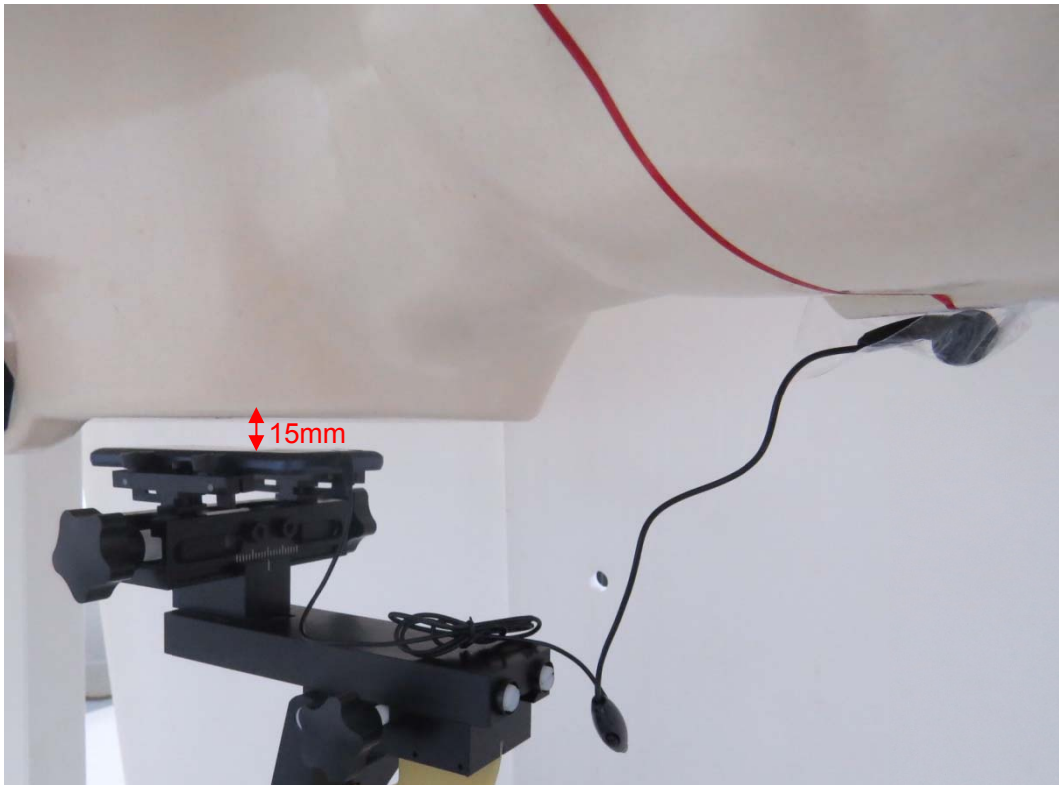
Picture 26: Back Side with Earphone, the distance from handset to the bottom of the Phantom is 15mm
