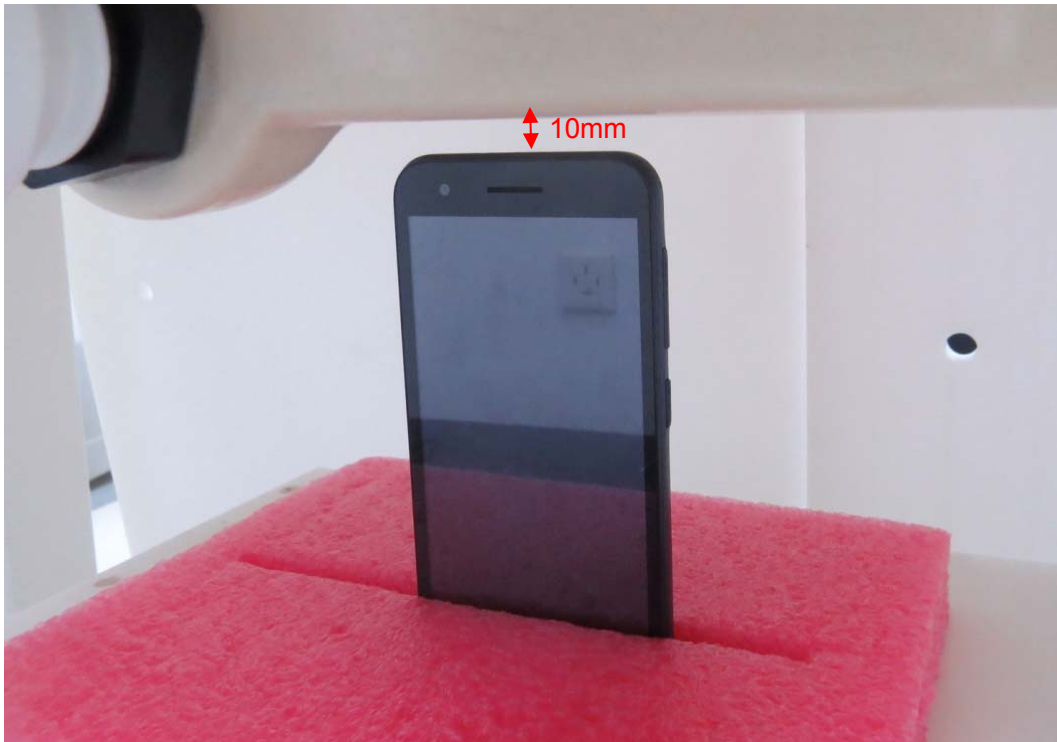
Picture 24: Top Side, the distance from handset to the bottom of the Phantom is 10mm
