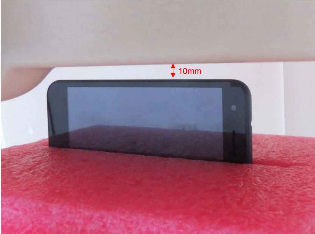
Picture 22: Left Side, the distance from handset to the bottom of the Phantom is 10mm
