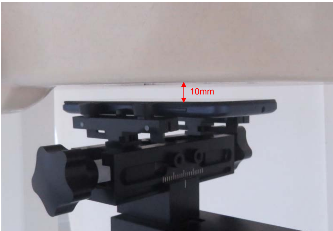
Picture 21: Front Side, the distance from handset to the bottom of the Phantom is 10mm
