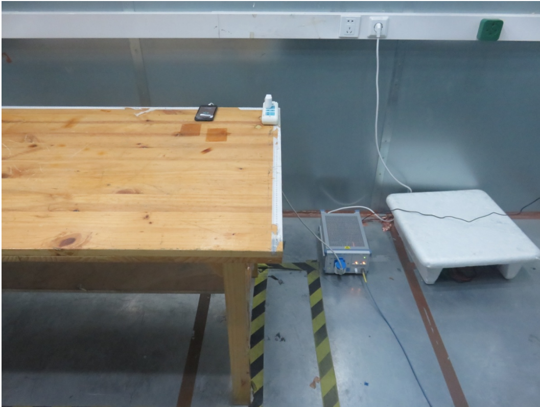
Picture 3 Conducted Emission Test Setup
