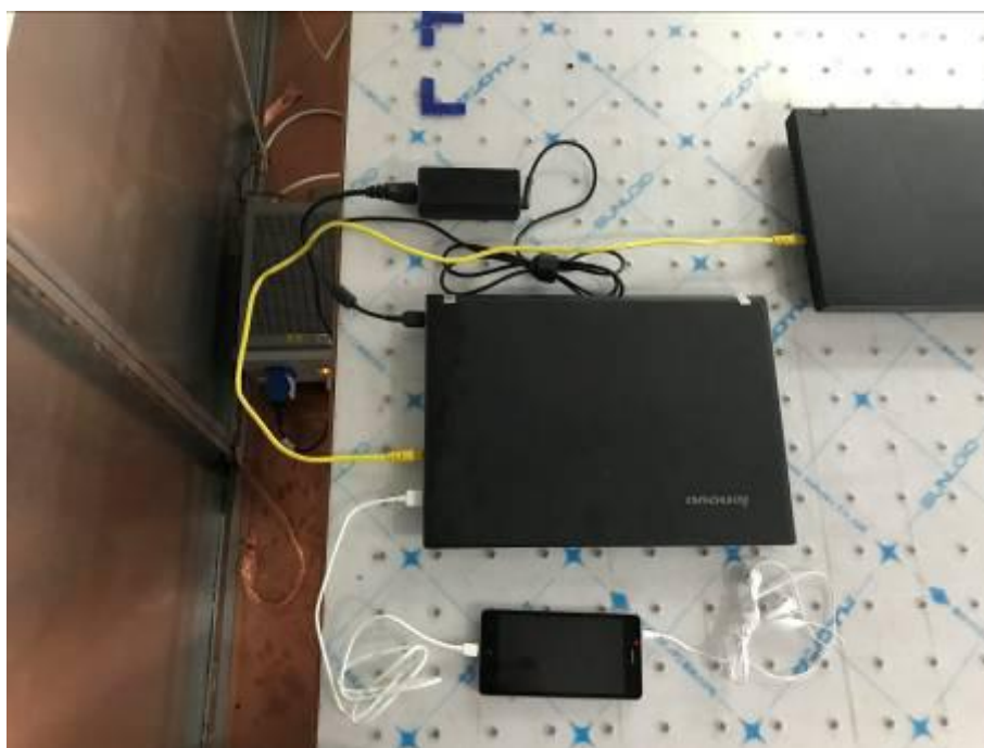
Conducted Emissions Test Setup (with laptop)
