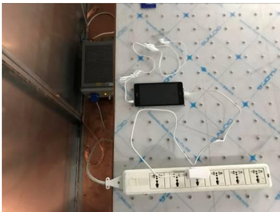
Conducted Emissions Test Setup (with charger)
