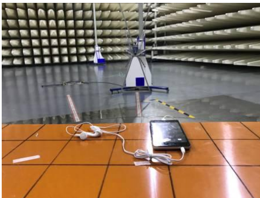
Radiated Emissions Test Setup (with charger)
