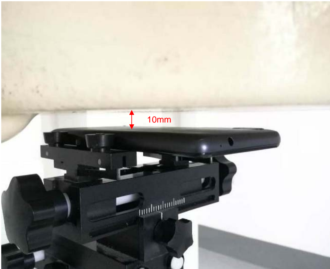
Picture 5: Back Side, the distance from handset to the bottom of the Phantom is 10mm
