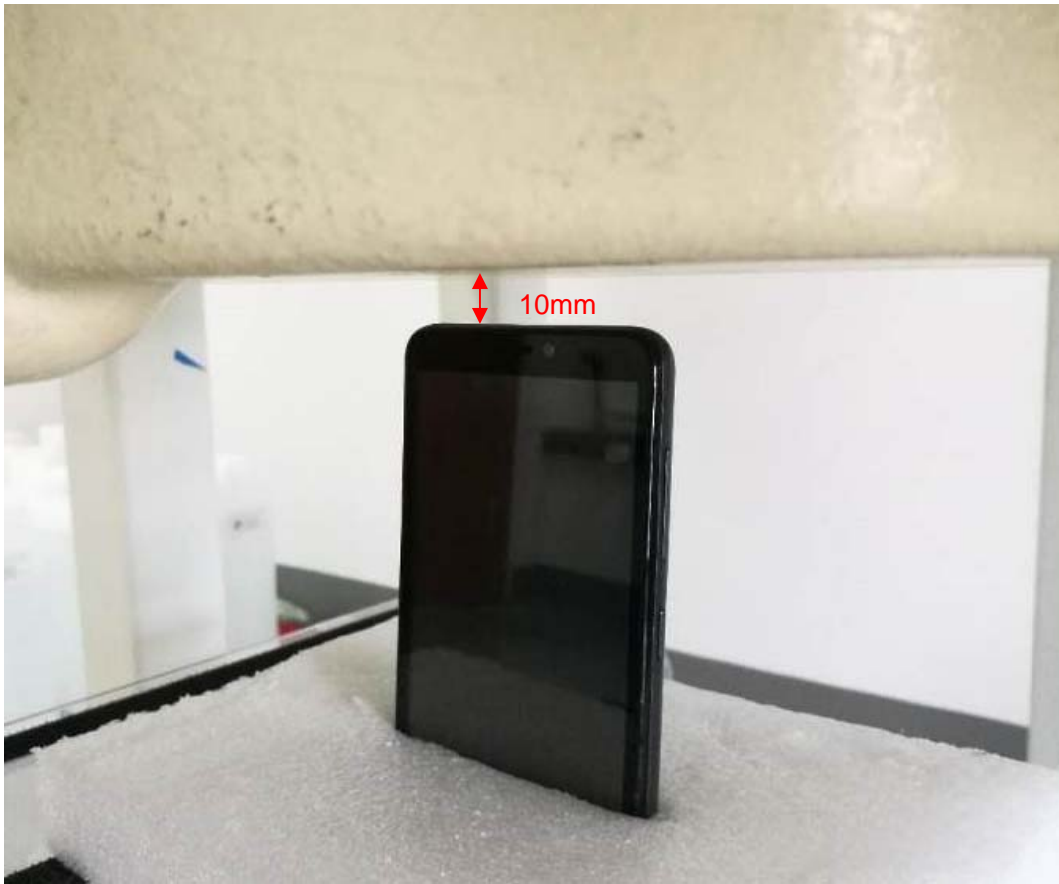
Picture 9: Top Side, the distance from handset to the bottom of the Phantom is 10mm
