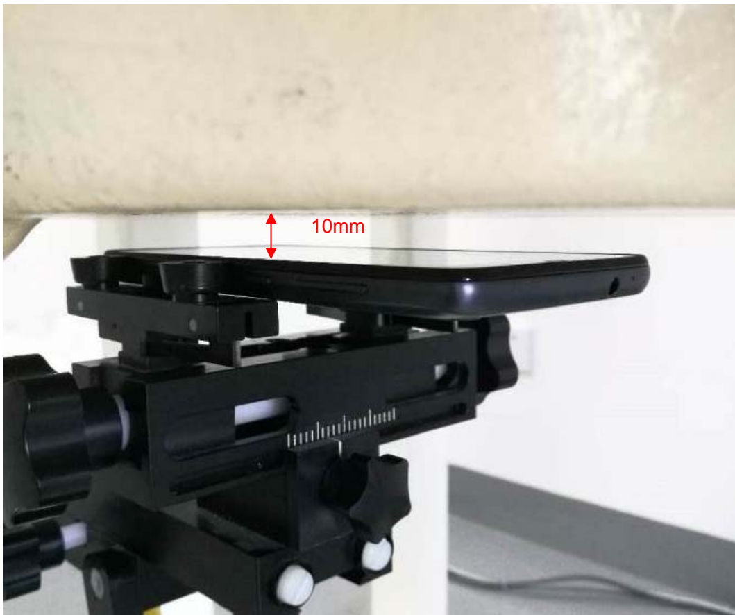
Picture 6: Front Side, the distance from handset to the bottom of the Phantom is 10mm
