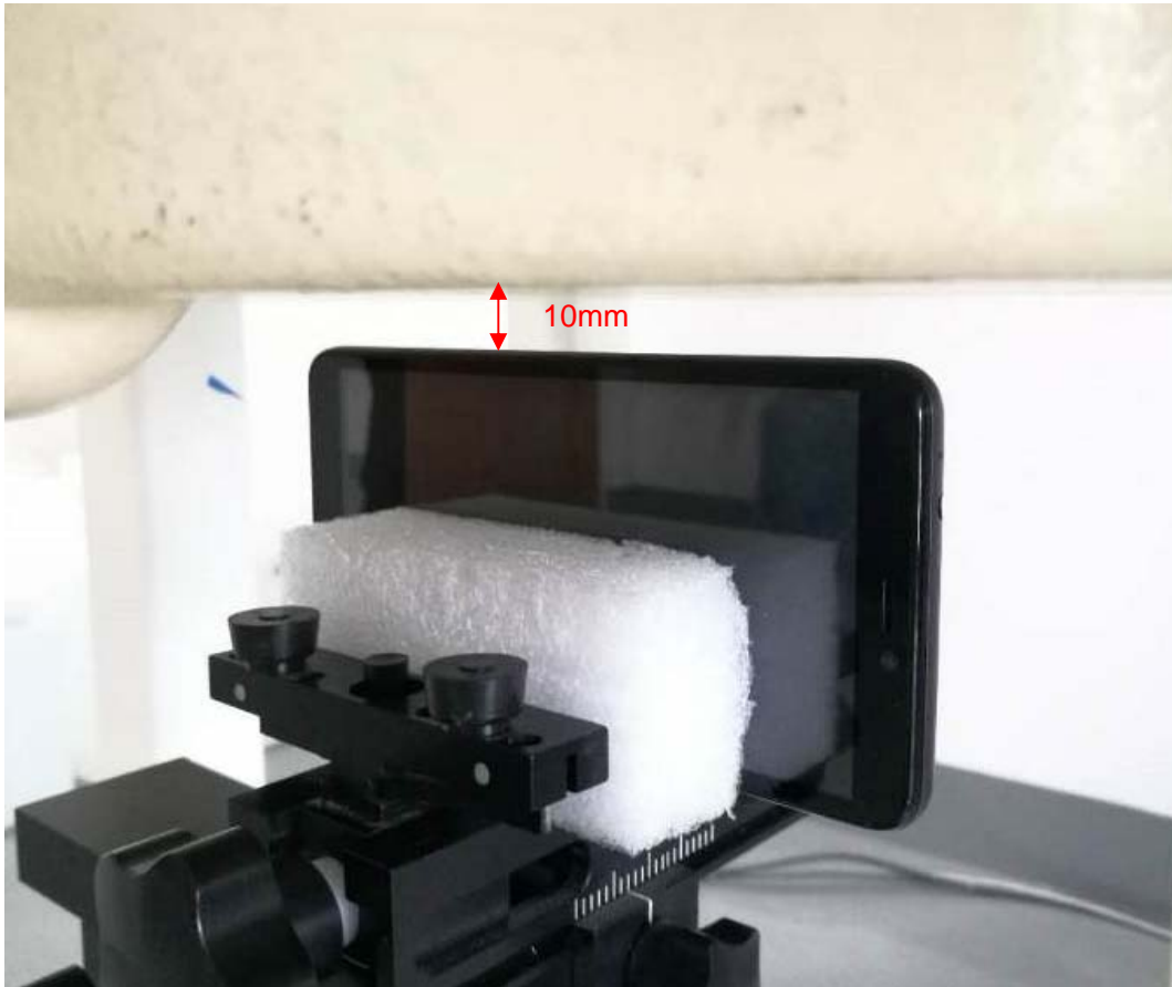
Picture 7: Left Side, the distance from handset to the bottom of the Phantom is 10mm
