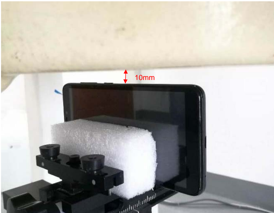
Picture 8: Right Side, the distance from handset to the bottom of the Phantom is 10mm
