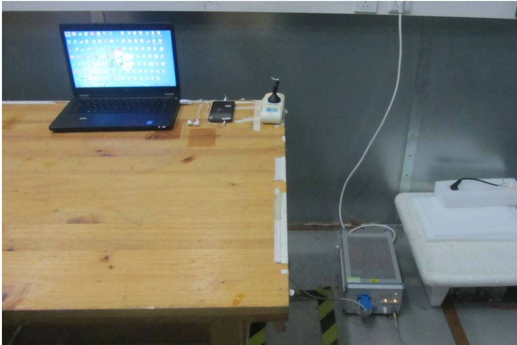
Picture 2 Conducted Emission Test Setup
