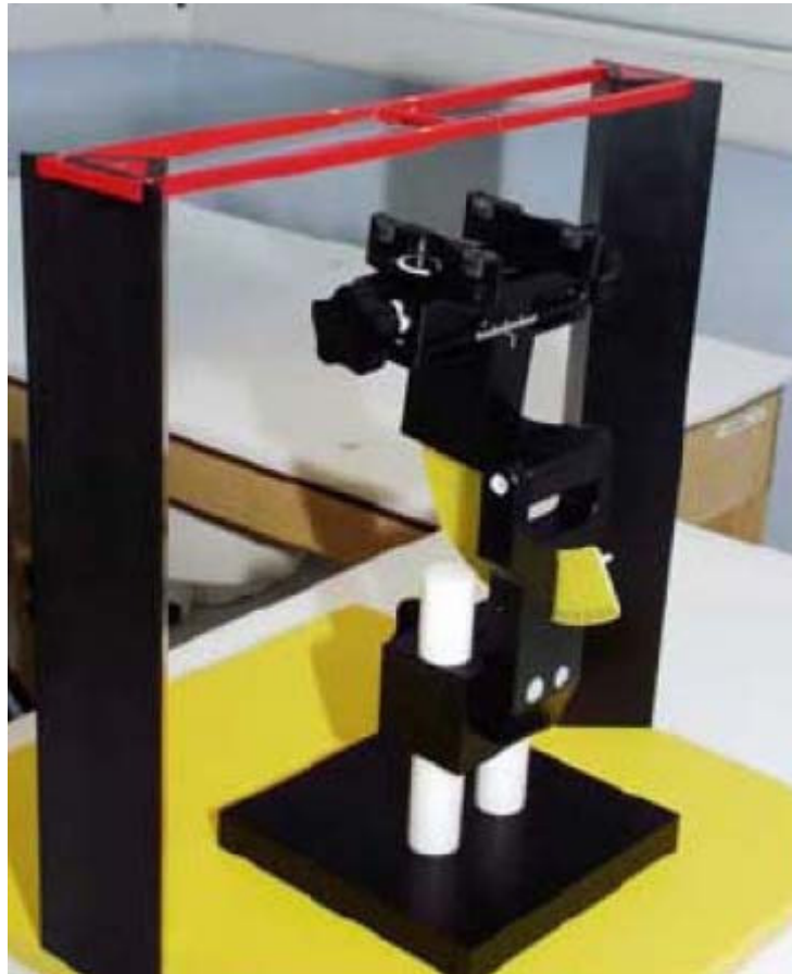
Figure 7 T-coil Phantom & Device Holder
