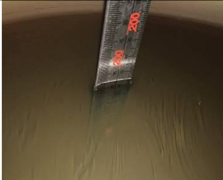
Liquid depth for SAR Measurement
