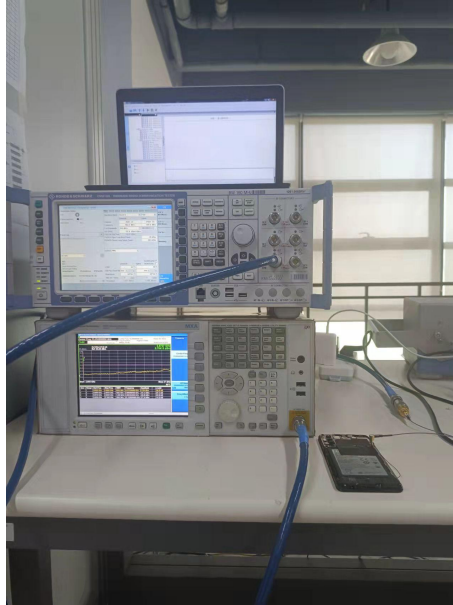
'RF Conducted Test setup (GSM/WCDMA/LTE)
