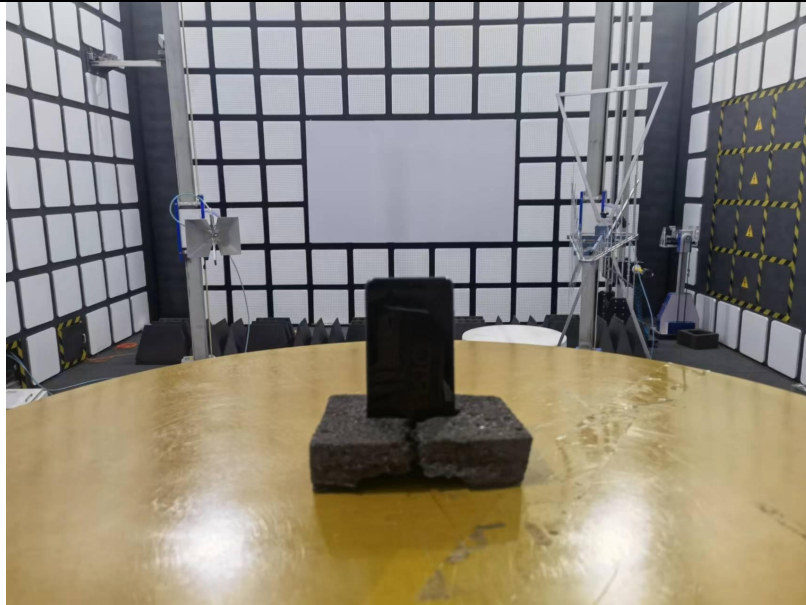
Spurious Radiated Emissions Test setup
