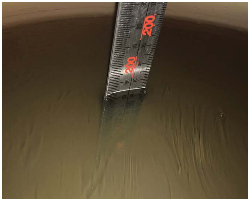
Liquid depth for SAR Measurement
