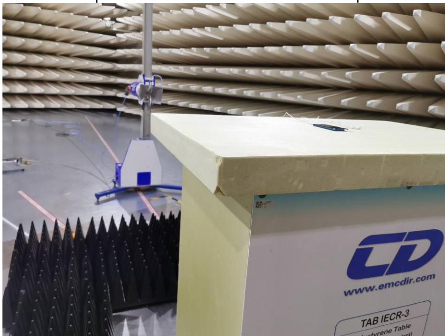
Spurious Radiated Emissions Test setup
