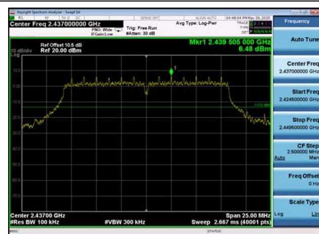
,Plot 1,Reference Level-802.11g ,2437MHz,Ant0
