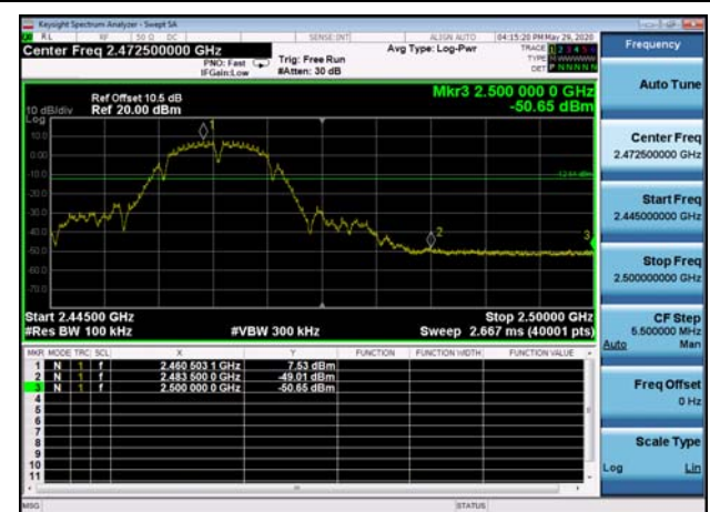
,Plot 2,Band Edge-802.11b,2462MHz ,Ant0
