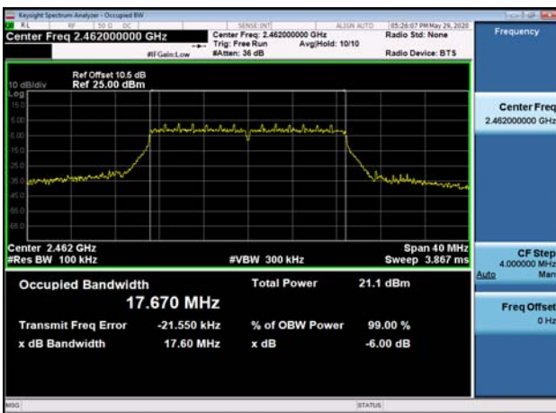
6dB Bandwidth-802.11n(HT20),2462MHz ,Ant0
