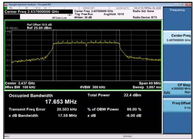
6dB Bandwidth-802.11n(HT20),2437MHz ,Ant0
