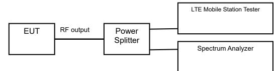
Test procedure: KDB 971168 D01 v03r01 – Section 6.0
