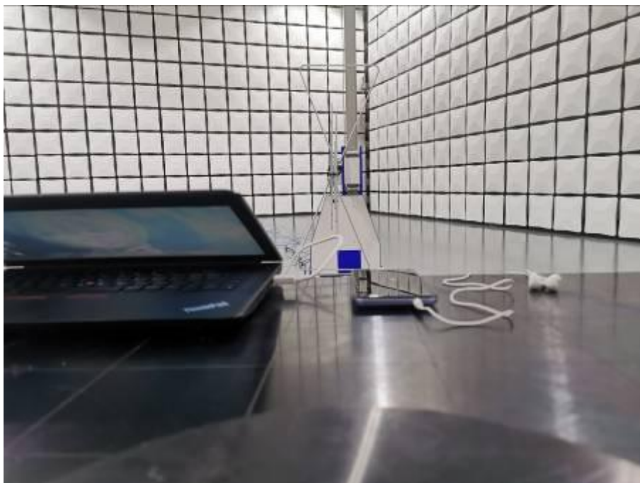
Radiated Emissions Test Setup (with laptop) (30-1000MHz)
