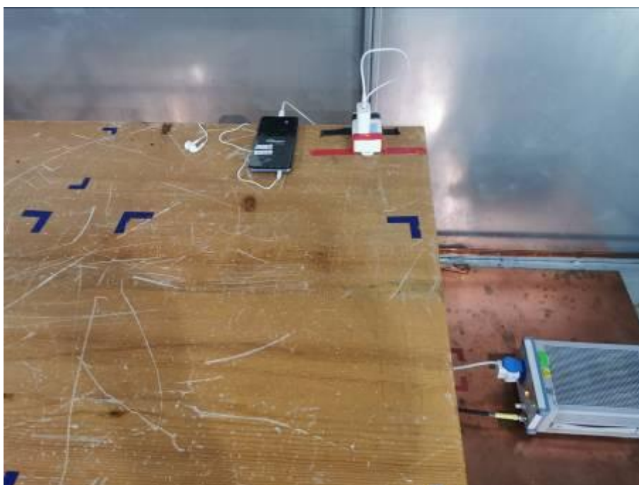
Conducted Emissions Test Setup (with charger)
