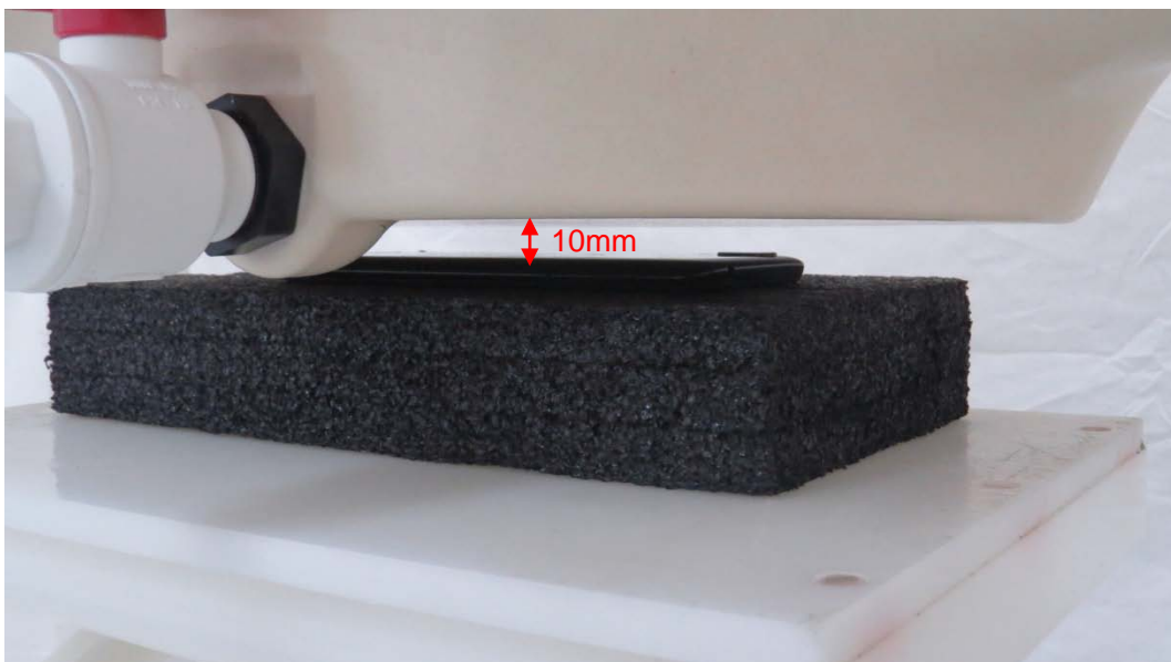
Picture 10: Back Side, the distance from handset to the bottom of the Phantom is 10mm
