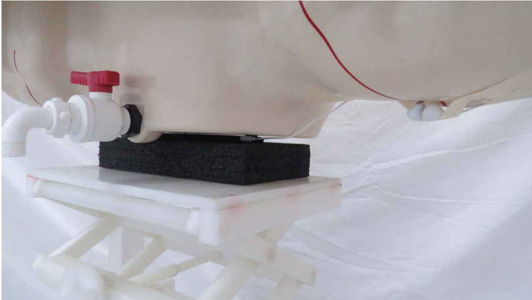
Picture 17: Back Side, the distance from handset to the bottom of the Phantom is 0mm with earphone
