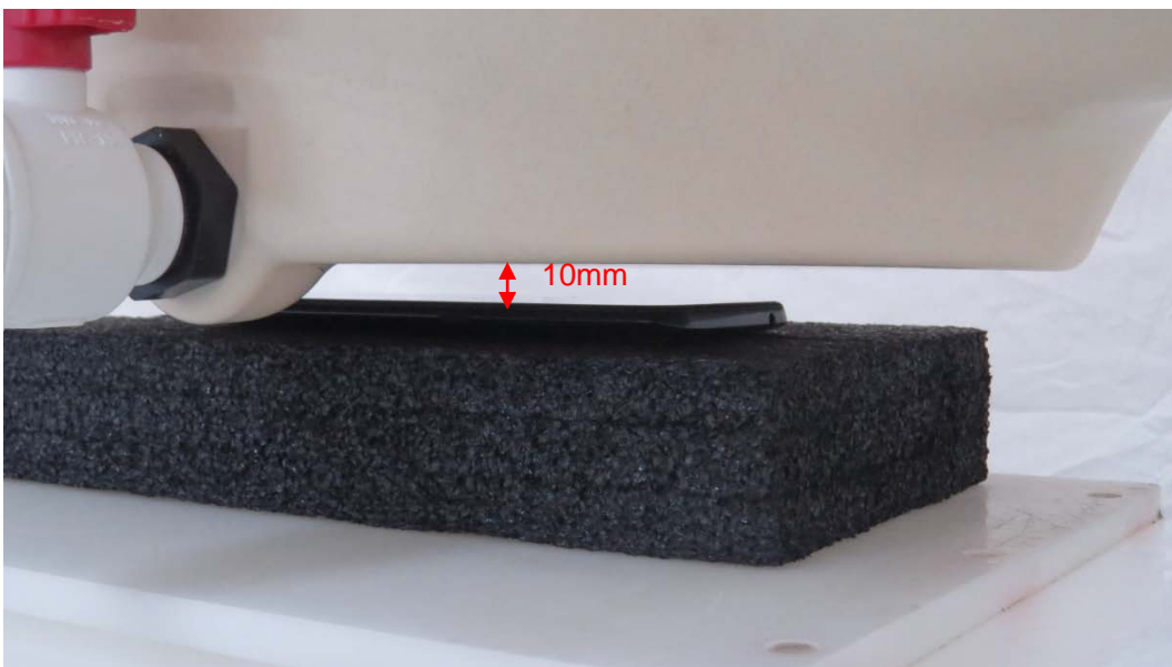
Picture 12: Front Side, the distance from handset to the bottom of the Phantom is 10mm
