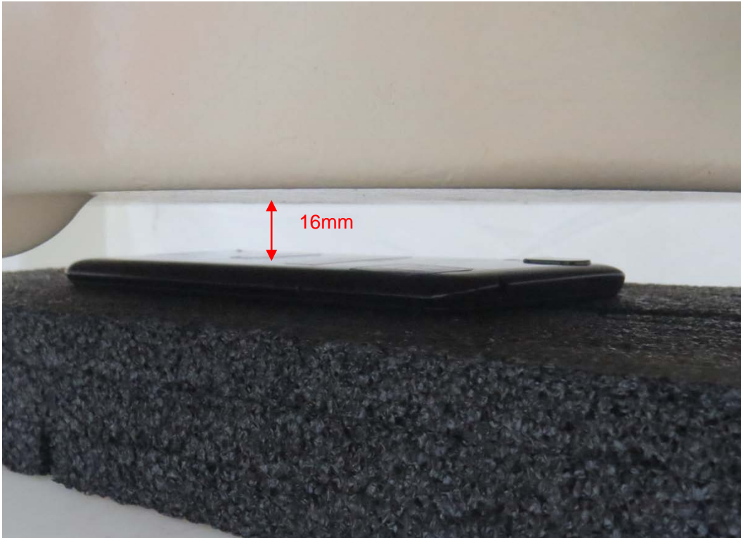
Picture 5: Back Side, the distance from handset to the bottom of the Phantom is 16mm
