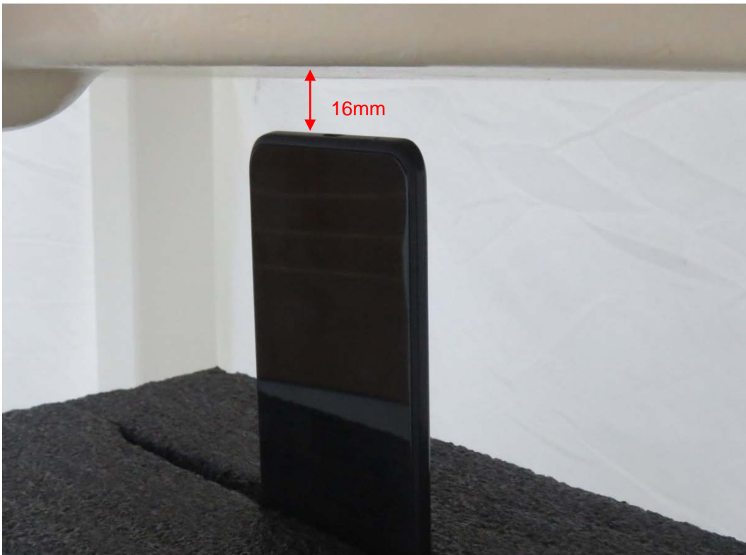
Picture 6: Bottom Edge, the distance from handset to the bottom of the Phantom is 16mm
