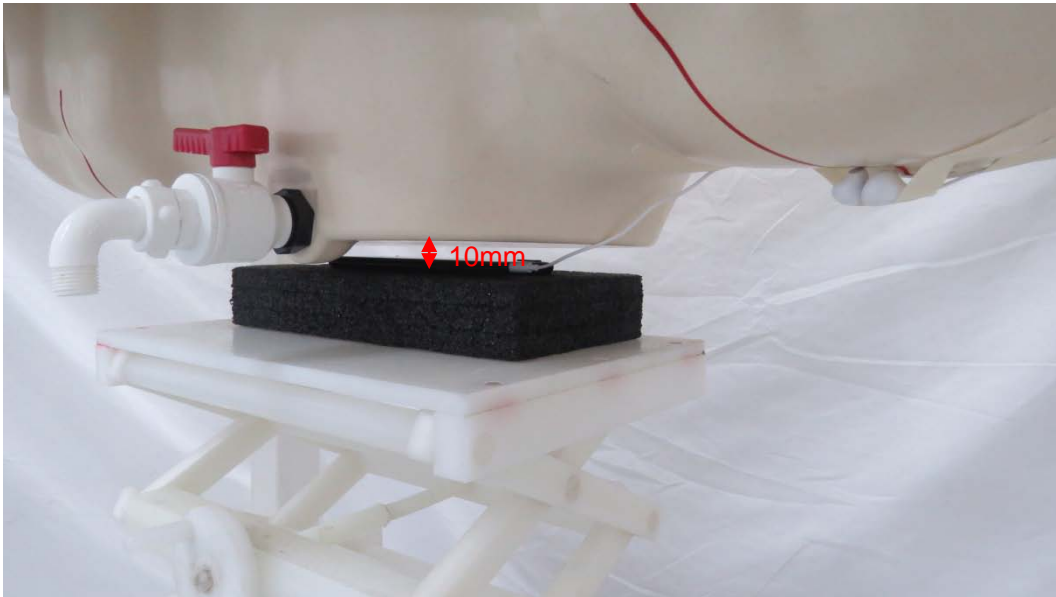
Picture 11: Back Side, the distance from handset to the bottom of the Phantom is 10mm with earphone
