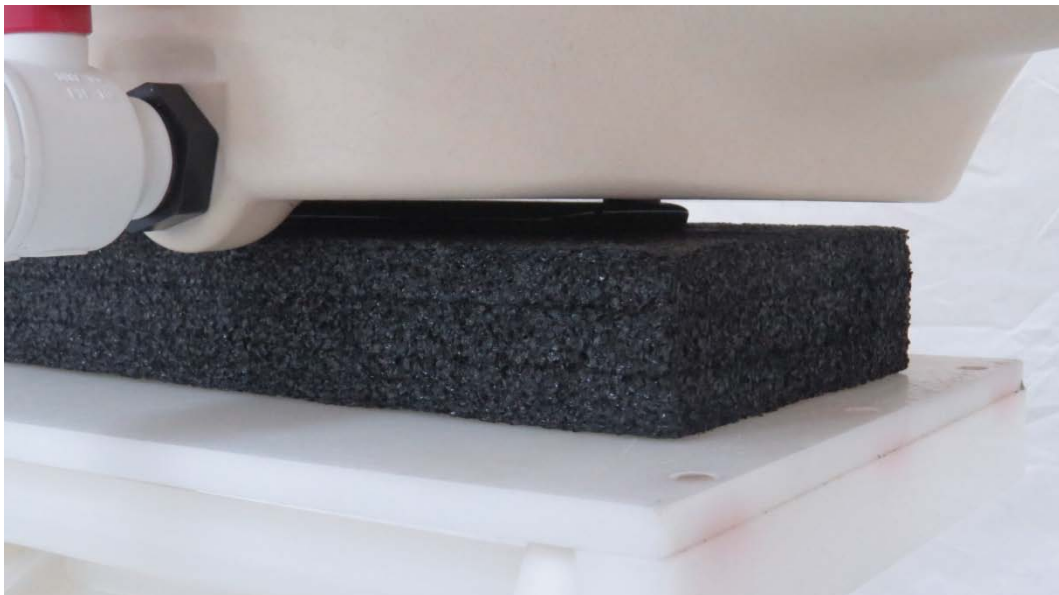
Picture 16: Back Side, the distance from handset to the bottom of the Phantom is 0mm
