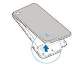
2. Insert the nano-SIM card into the right card slot, and insert the microSDXC card (optional) into the left card slot.
