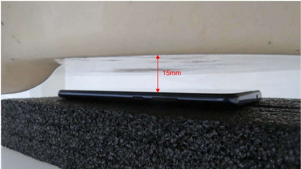
Picture 6: Front Side, the distance from handset to the bottom of the Phantom is 15mm
