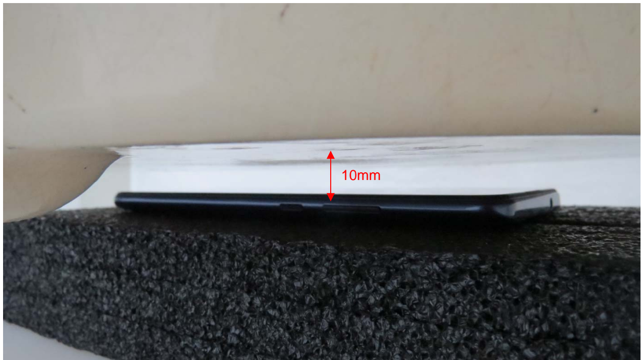
Picture 8: Front Side, the distance from handset to the bottom of the Phantom is 10mm
