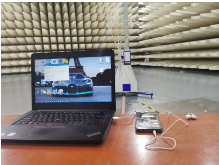
Radiated Emissions Test Setup (with laptop) (30-1000MHz)
