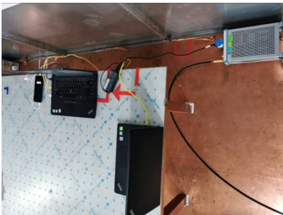
Conducted Emissions Test Setup (with laptop)
