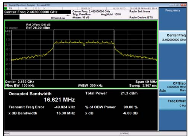
6dB Bandwidth-802.11g,2462MHz
