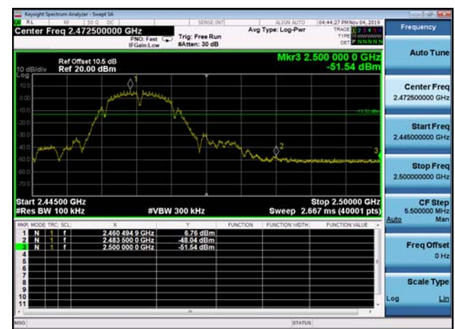
,Plot 2,Band Edge-802.11b,2462MHz
