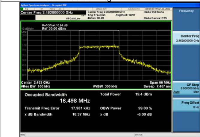
Test Mode:802.11g 2462MHz Chain0
