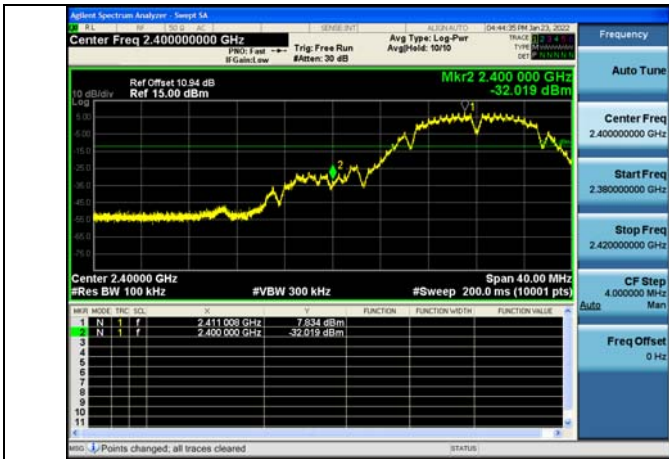
Test Mode:802.11b 2412MHz Chain0
