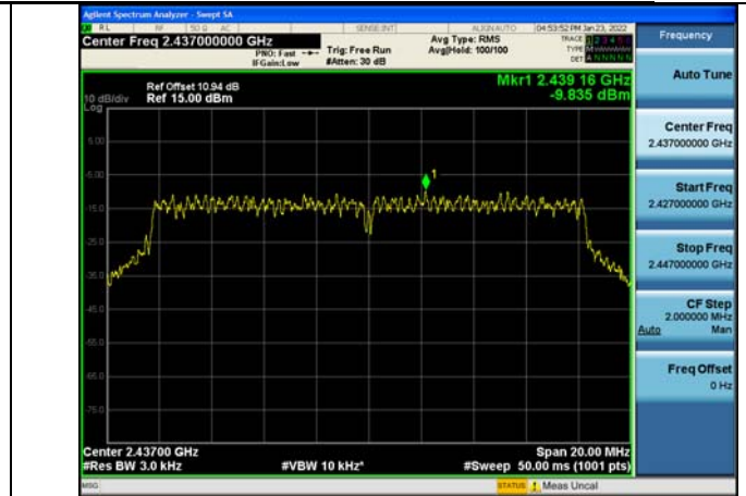
Test Mode:802.11g 2437MHz Chain0
