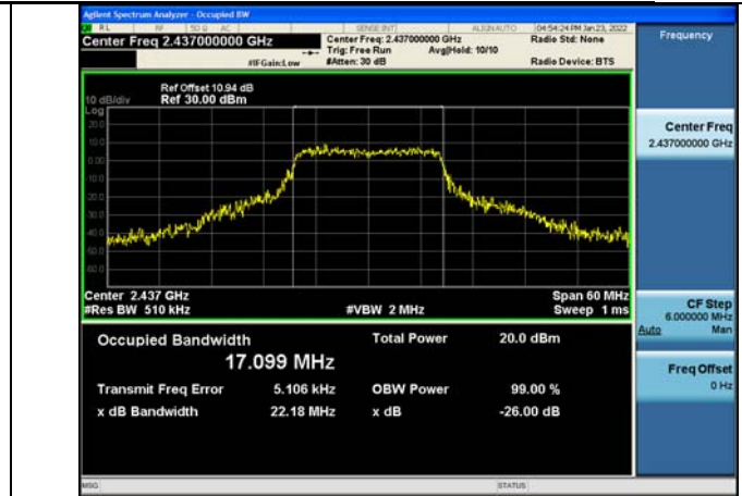
Test Mode:802.11g 2437MHz Chain0
