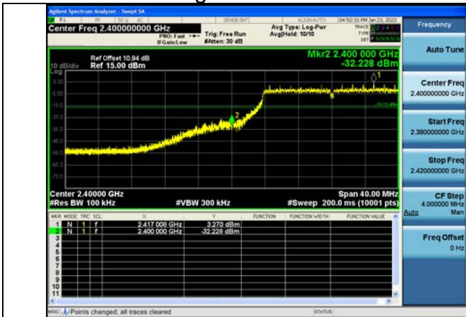
Test Mode:802.11g 2412MHz Chain0
