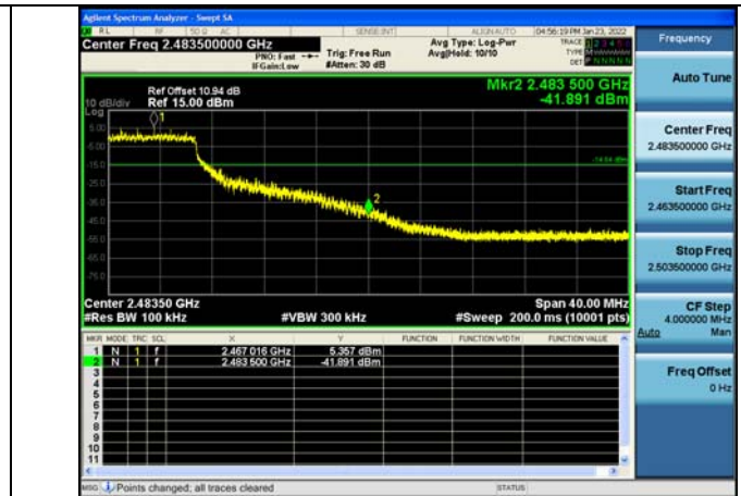
Test Mode:802.11g 2462MHz Chain0
