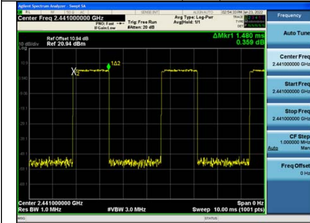
Test Mode: \pi/4 DQPSK(2DH5) 2441MHz
