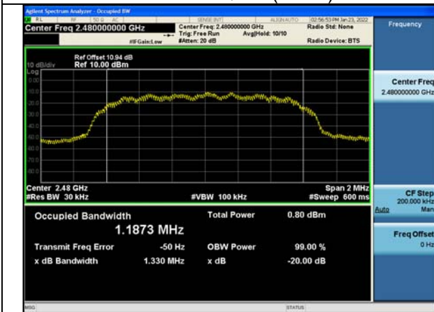
Test Mode:π/4QPSK(2DH5) MHz
