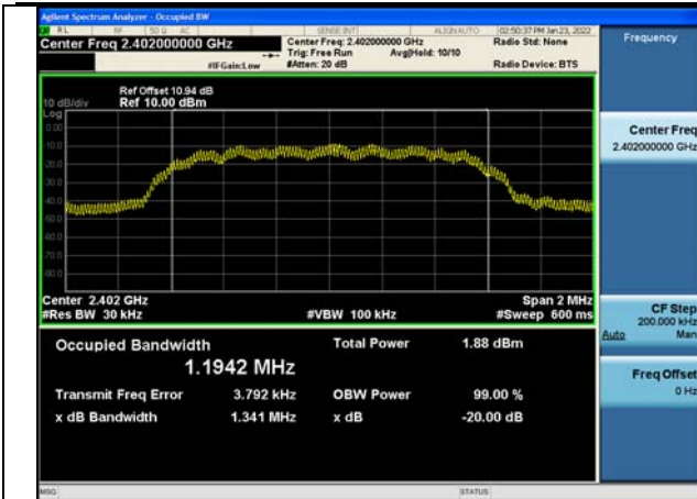
Test Mode:π/4QPSK(2DH5) MHz
