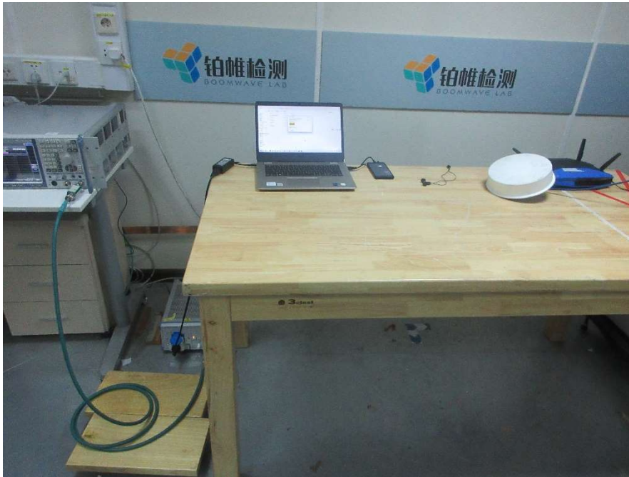
Conducted Emission 150kHz-30MHz (Front view) – Mode 5
