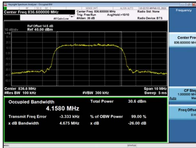
(Plot E2: WCDMA 850MHz Channel = 4183 Occupied bandwidth)
