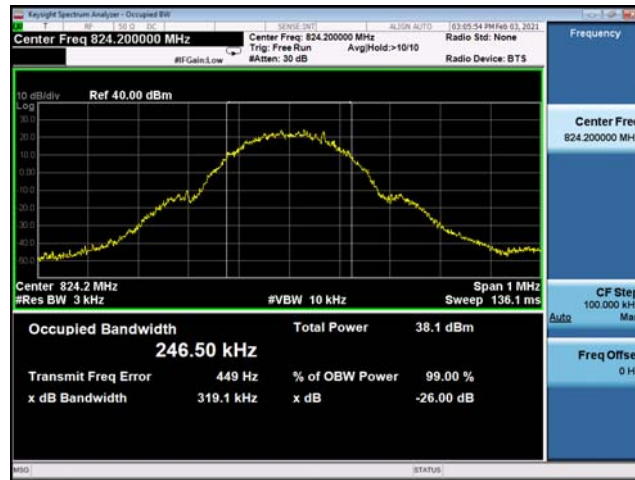
(Plot A1: GSM 850MHz Channel = 128 Occupied bandwidth)
