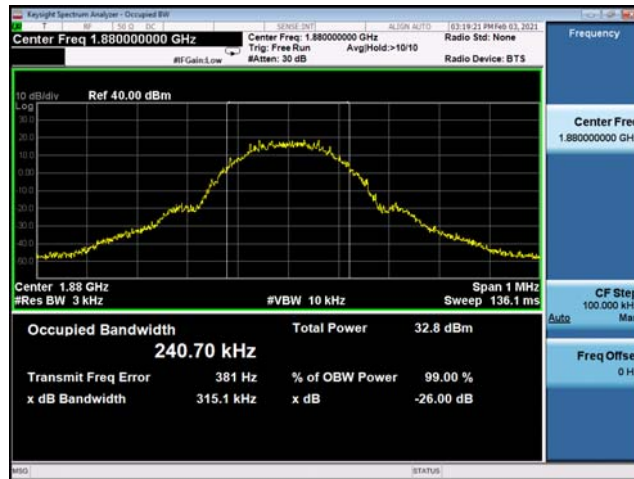
(Plot D2: EDGE 1900MHz Channel = 661 Occupied bandwidth)
