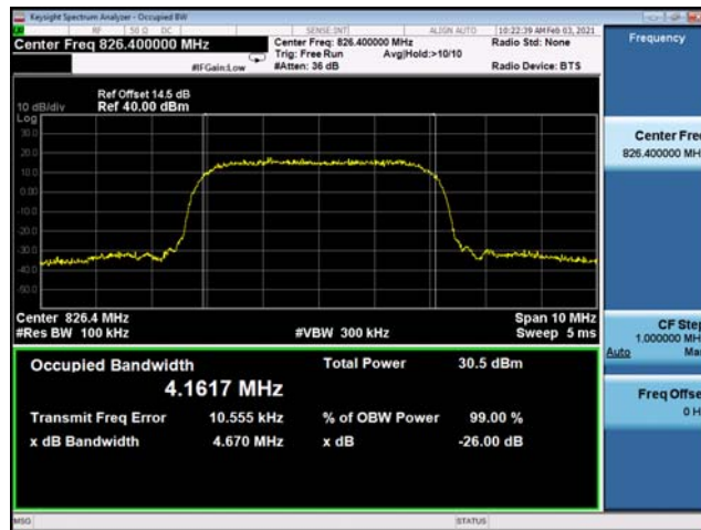
(Plot E1: WCDMA 850MHz Channel = 4132 Occupied bandwidth)
