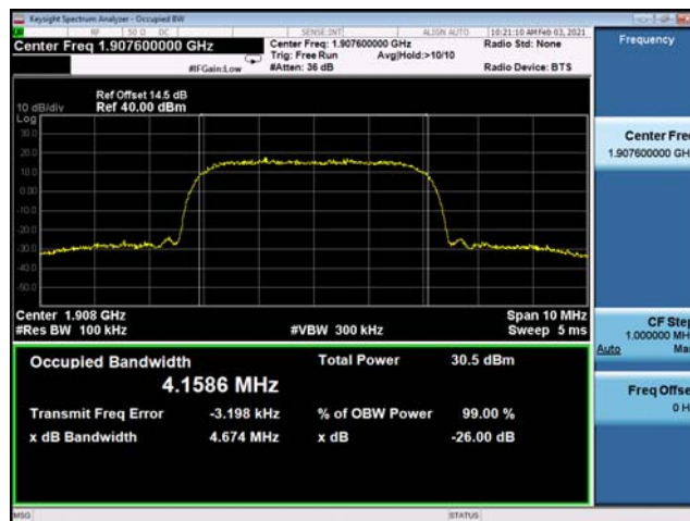
(Plot F3: WCDMA 1900MHz Channel = 9538 Occupied bandwidth)
