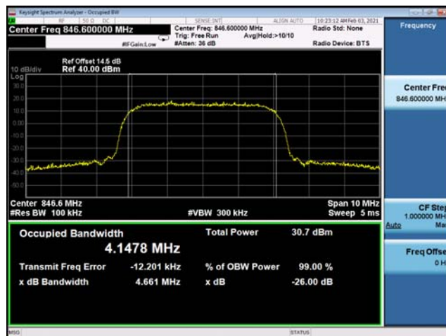
(Plot E3: WCDMA 850MHz Channel = 4233 Occupied bandwidth)
