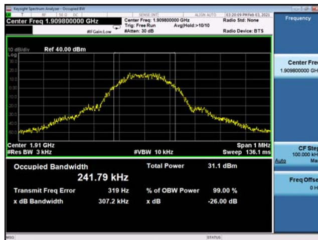
(Plot D3: EDGE 1900MHz Channel = 810 Occupied bandwidth)
