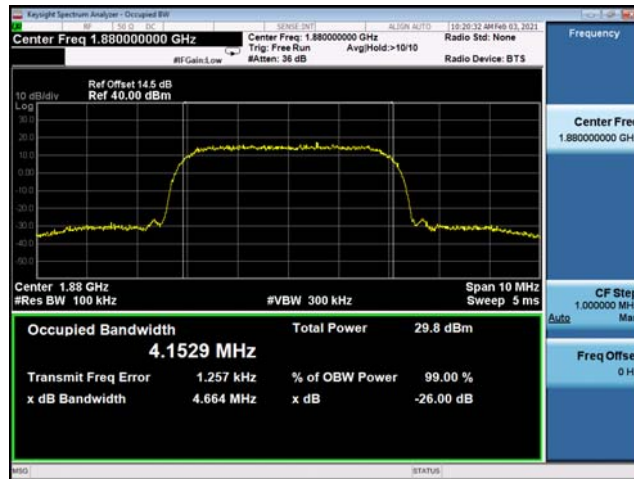
(Plot F2: WCDMA 1900MHz Channel = 9400 Occupied bandwidth)
