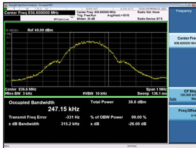
(Plot A2: GSM 850MHz Channel = 190 Occupied bandwidth)
