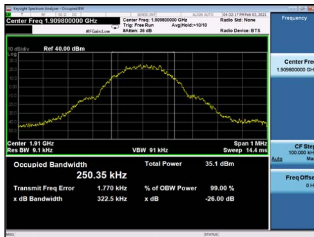
(Plot B3: GSM 1900MHz Channel = 810 Occupied bandwidth)
