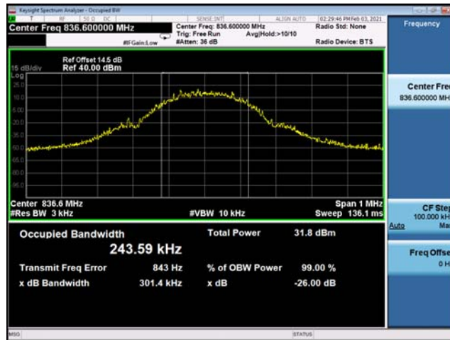
(Plot C2: EDGE 850MHz Channel = 190 Occupied bandwidth)
