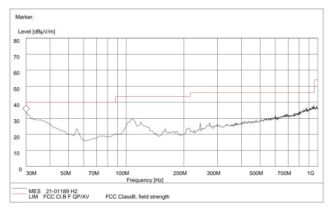
Plot A: 30MHz to 1GHz, Antenna Horizontal
