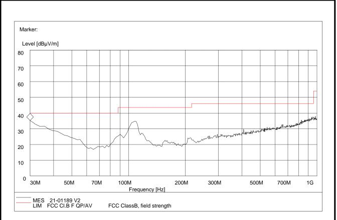
Plot B: 30MHz to 1GHz, Antenna Vertical
