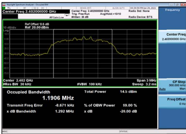
20dB Bandwidth: 8DPSK,2480MHz,3DH5
