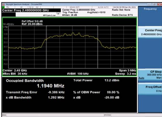
20dB Bandwidth: 8DPSK,2480MHz,3DH5
