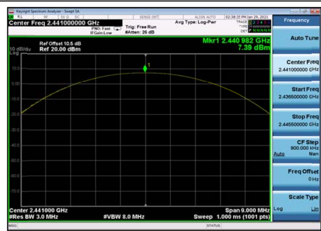
Output Power: DQPSK,2402MHz,2DH5
