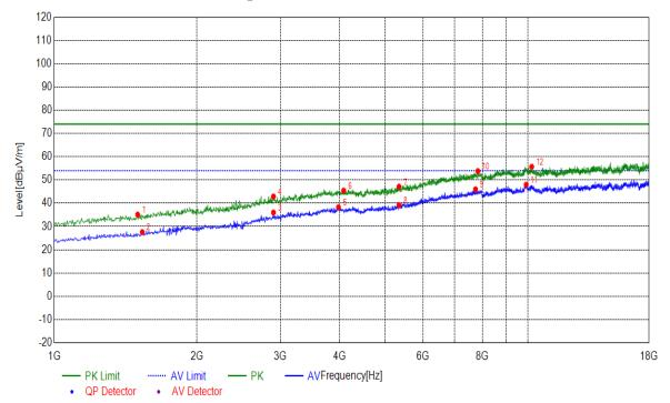
(Plot E: Test Antenna Horizontal 1G – 18G)
