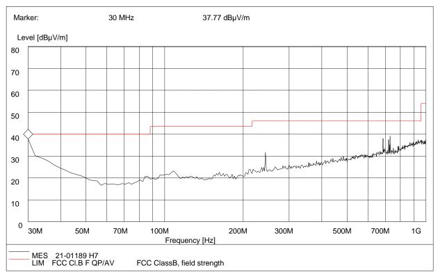
(Plot D: Test Antenna Horizontal 30M - 1G)
