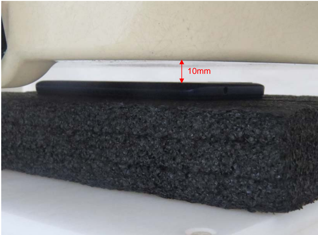
Picture 7: Back Side, the distance from handset to the bottom of the Phantom is 10mm
