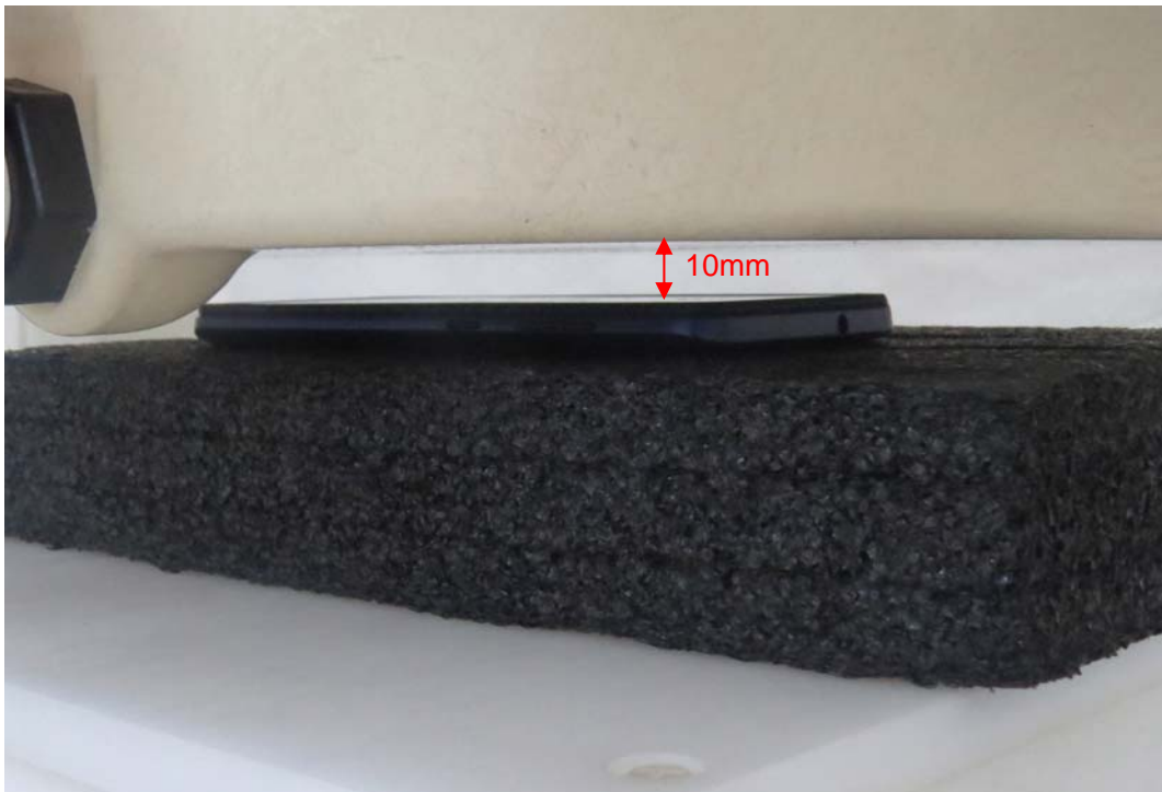
Picture 8: Front Side, the distance from handset to the bottom of the Phantom is 10mm
