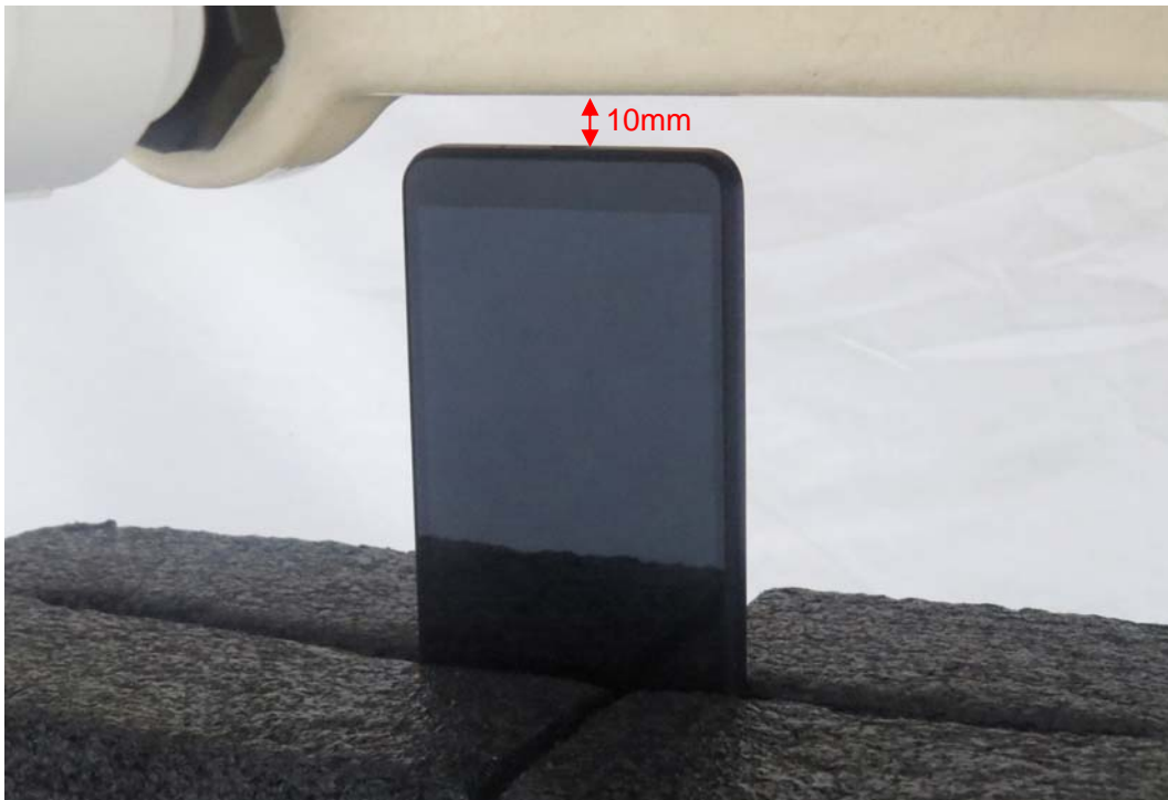
Picture 12: Bottom Edge, the distance from handset to the bottom of the Phantom is 10mm
