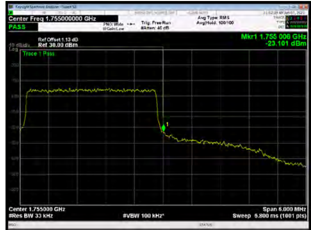
LTE Band 4 QPSK 5MHz CH-High, 1 RB
