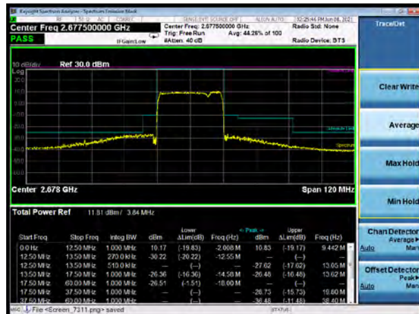
CA_41C 16QAM 20MHz+5MHz CH- High, RB 1
