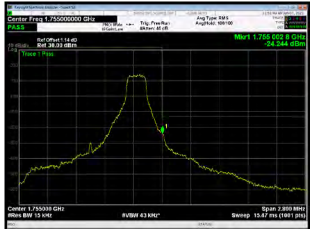
LTE Band 4 QPSK 1.4MHz CH-High, 100%RB
