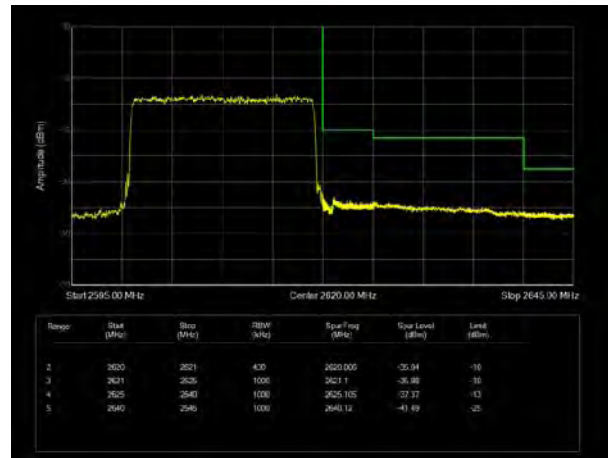
LTE Band 38 64QAM 20MHz CH-High, 100%RB
