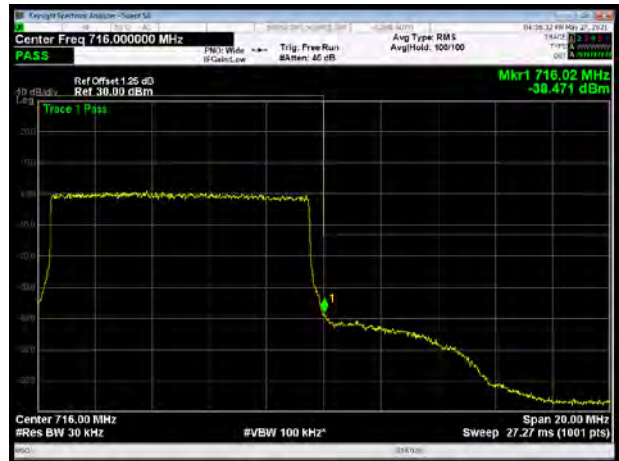
LTE Band 12 16QAM 1.4MHz CH-High, 1 RB
