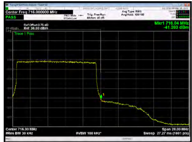
LTE Band 17 64QAM 10MHz CH-High, 100%RB
