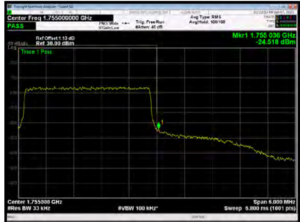
LTE Band 4 64QAM 5MHz CH-High, 1 RB
