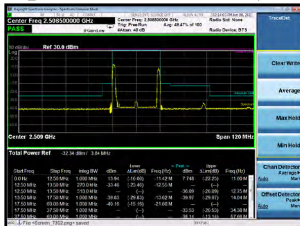
CA_41C 64QAM 20MHz+5MHz CH-Low, 100%RB
