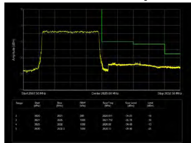
LTE Band 38 16QAM 10MHz CH-High, 100%RB
