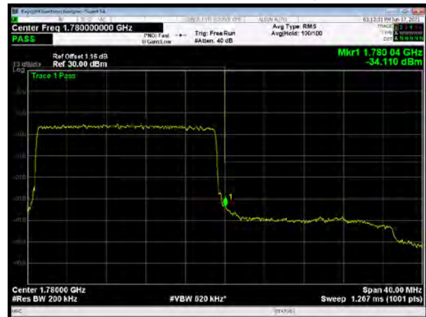
LTE Band 66 QPSK 20MHz CH-High, 100%RB
