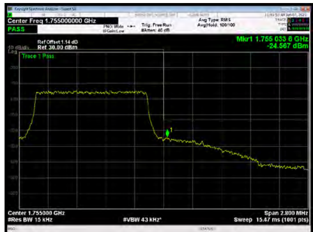
LTE Band 4 QPSK 3MHz CH-High, 1 RB
