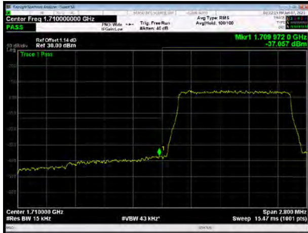
LTE Band 4 64QAM 3MHz CH-Low, 1 RB
