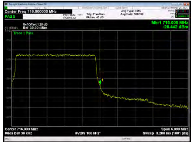
LTE Band 12 QPSK 5MHz CH-High, 1 RB
