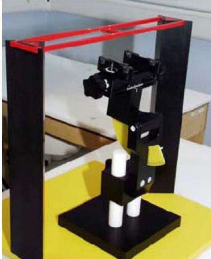
Figure 7 T-coil Phantom & Device Holder
